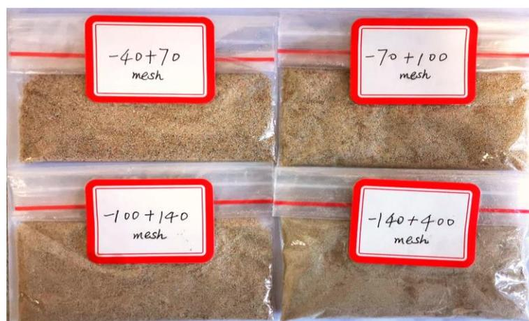
**Figure A1.** Quartz-sand picture of four fractions.
