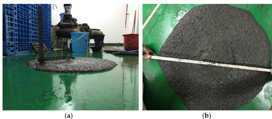
Figure 6. Slump and expansion tests: (a) slump, (b) expansion.
