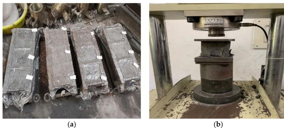
Figure 10. UCS tests: (a) sample preparation; (b) UCS test.
