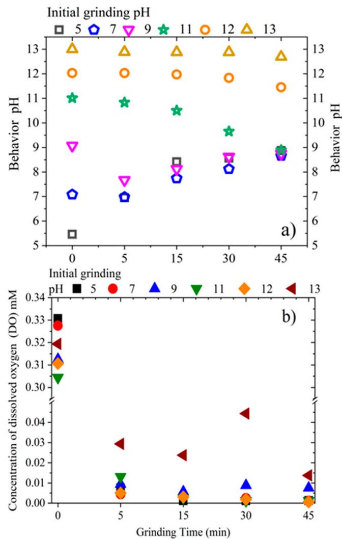
**Figure 1.** (a) pH behaviour as a function of grinding time (initial pH 5–13); (b) concentration of dissolved oxygen vs. grinding time (pH 5–13).
