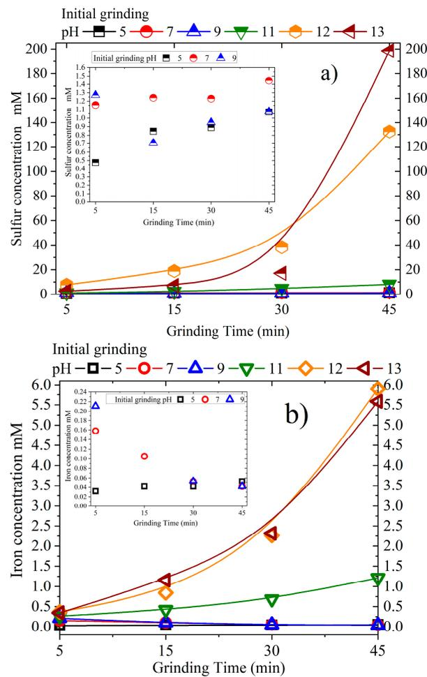
**Figure 2.** (a) Iron concentration (mM) as a function of grinding time (minutes); (b) sulphur concentration (mM) as a function of grinding time (minutes).
