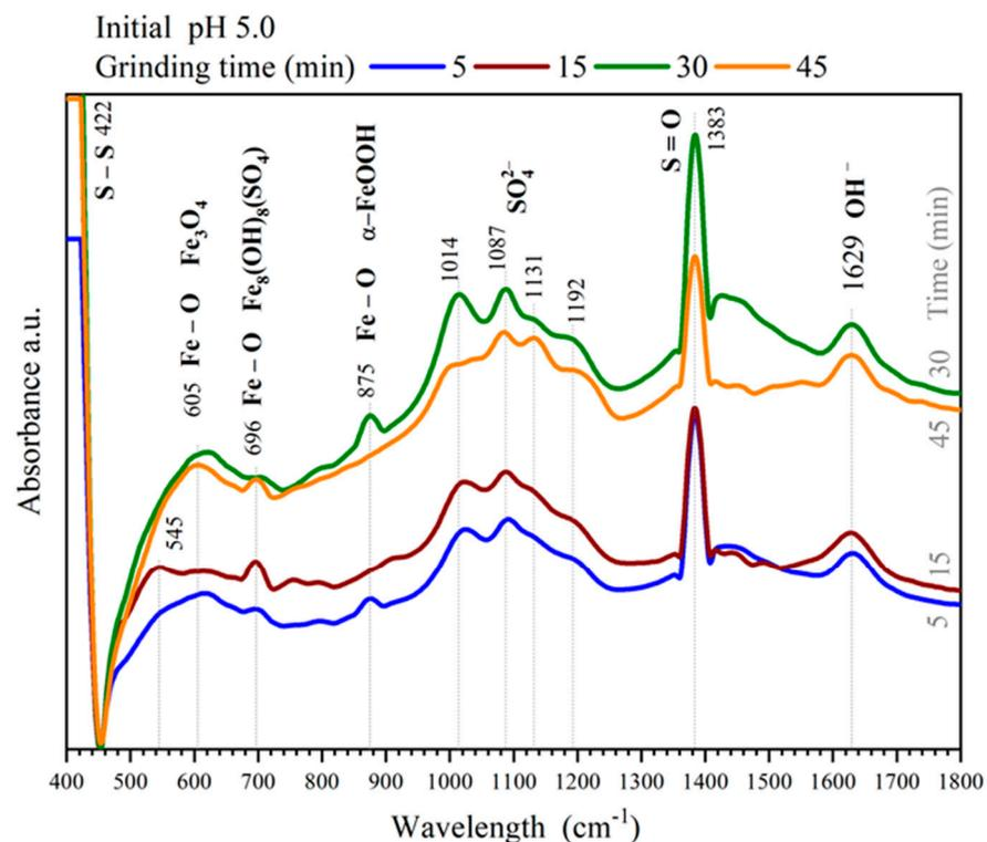
**Figure 6.** FT–IR spectra of pyrite ground with steel media at an initial pH of 5.0.
