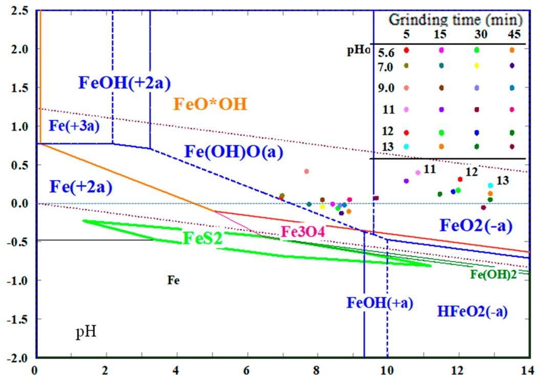
**Figure 3.** Eh–pH diagram of the Fe–S–H<sub>2</sub>O system at 25 °C and 1M. Recorded pulp potential values and pulp potential values vs. standard hydrogen electrode.
