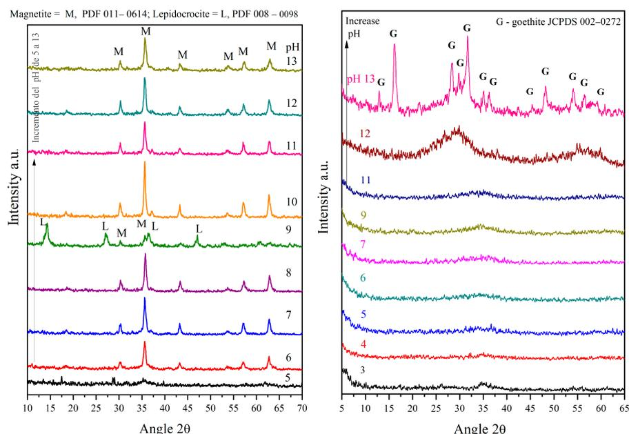
**Figure 11.** (a) Diffractograms of ferrous (+2) iron precipitates (2.86 mM concentration); (b) ferric (+3) iron precipitates (1.43 mM).
