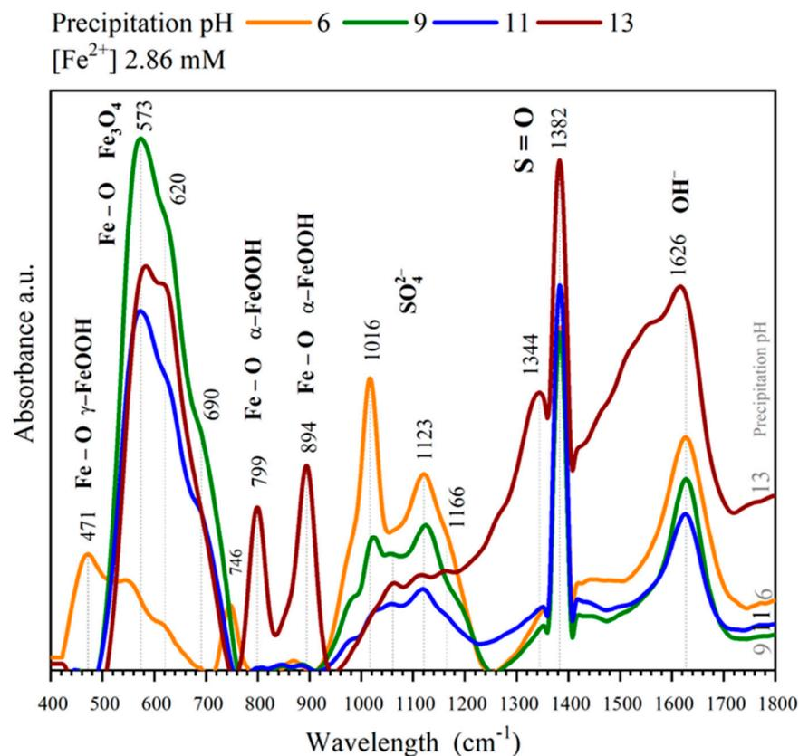
**Figure 13.** FT–IR spectra of the  $2.86 \text{ mM Fe (+2)}$  precipitates at  $\text{pH} = 6, 9, 11$  and  $13$ .
