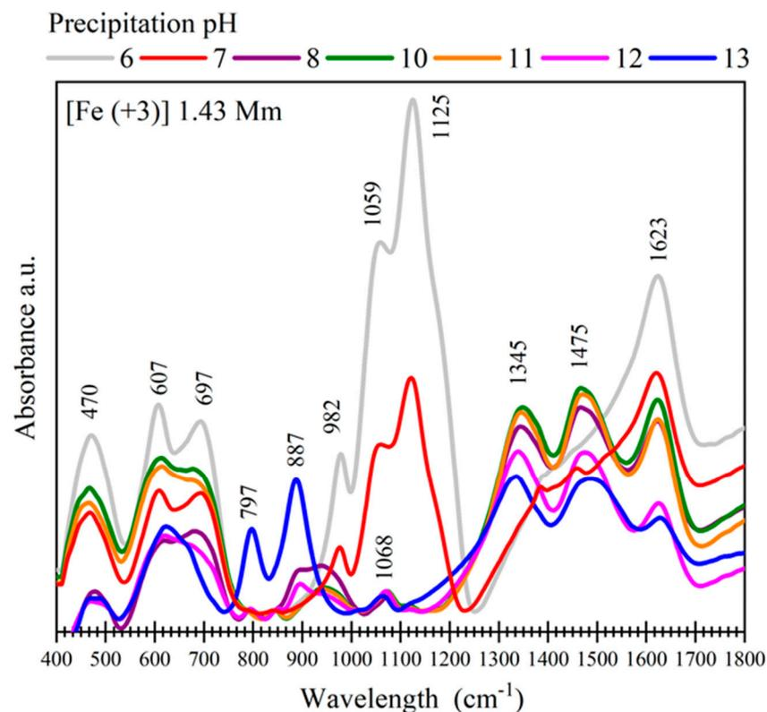
**Figure 12.** FT–IR spectra of the 1.43 mM Fe (+3) precipitates for the pH values 6, 7, 8, 10, 11, 12 and 13.
