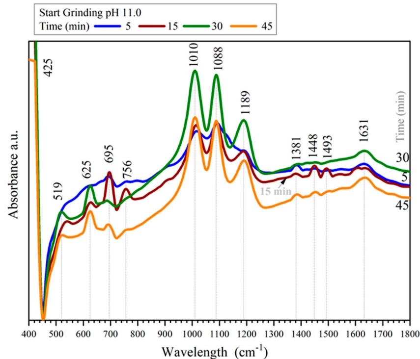
**Figure 8.** FT–IR spectra of pyrite ground with steel media (initial pH 11.0).
