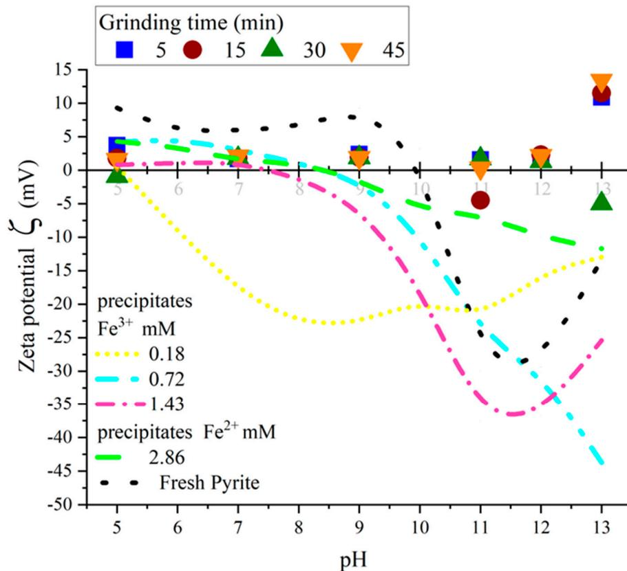
**Figure 5.** Zeta potential ( $\zeta$ : mV) against pH of pyrite obtained from grinding and fresh grinding and of ferric (0.18, 0.72 and 1.43 mM) and ferrous iron precipitates (2.86 mM).
