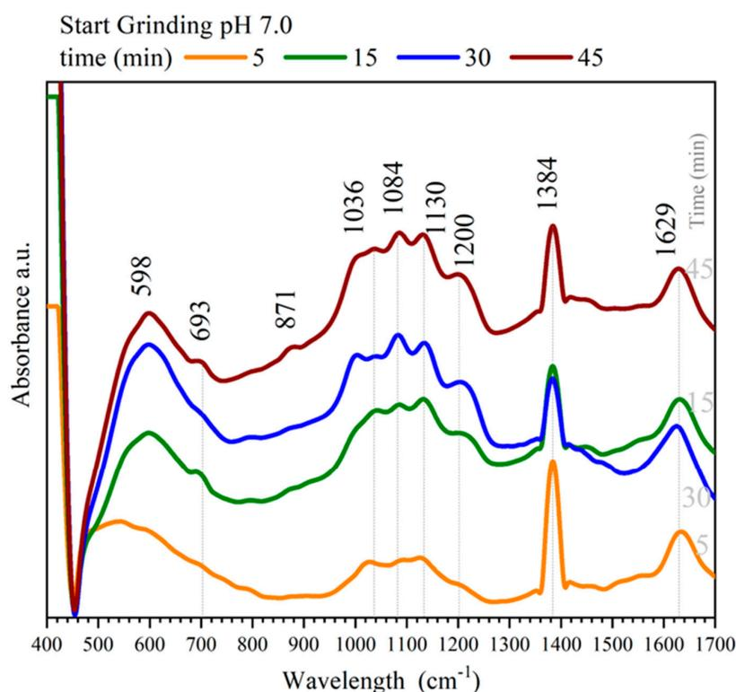
**Figure 7.** FT–IR spectra of pyrite ground with steel media (initial pH 7.0).
