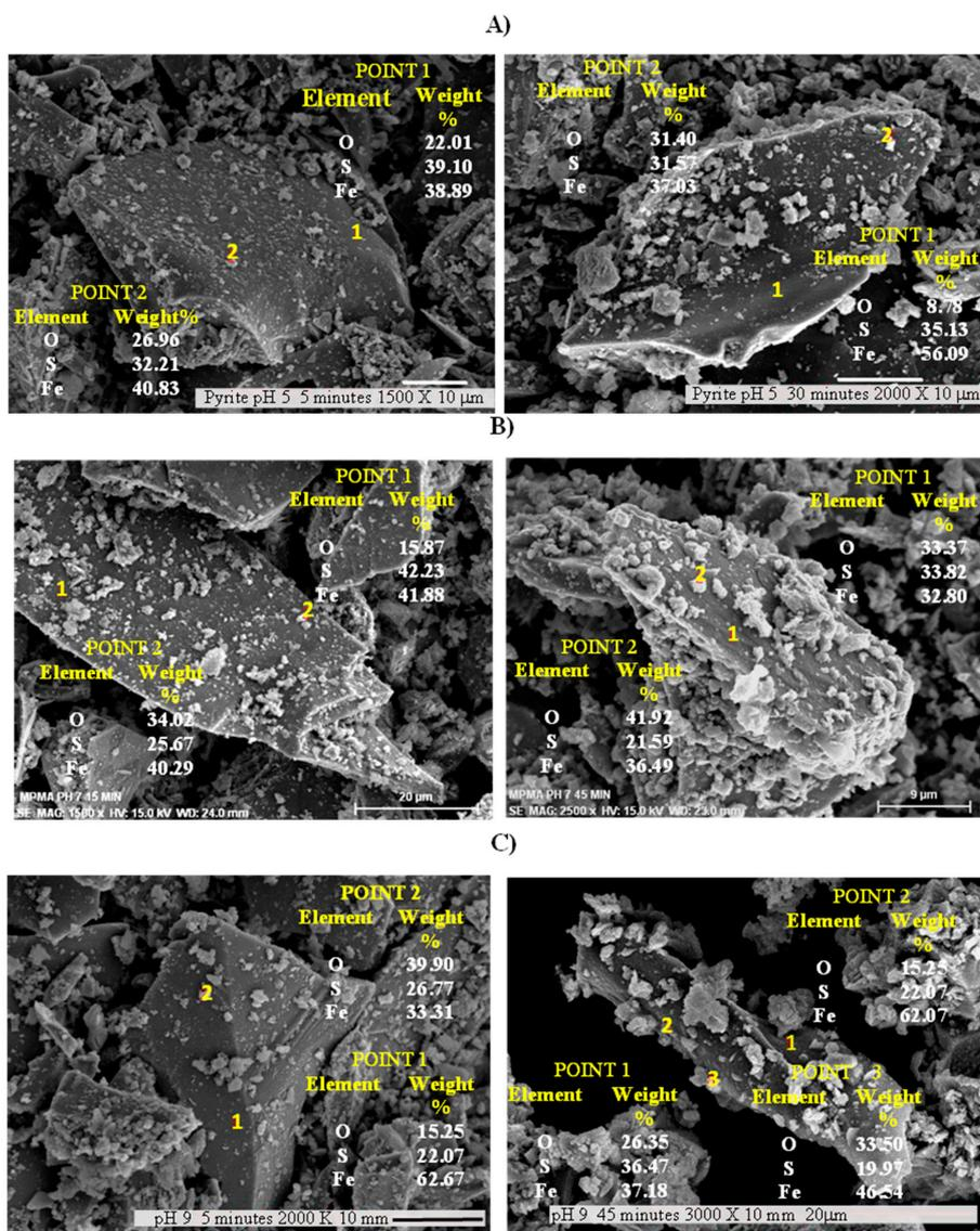
Figure 10. SEM-EDS micrographs of the pyrite particles obtained after grinding with steel media: initial pH 5 (A), 7 (B) and 9 (C).
