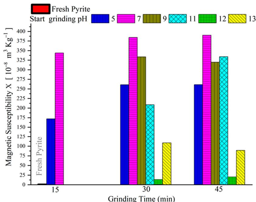
**Figure 9.** Specific magnetic susceptibility  $\chi \times 10^{-8} \text{ m}^3 \text{ Kg}^{-1}$  of the pyrite particles obtained from grinding with steel media.
