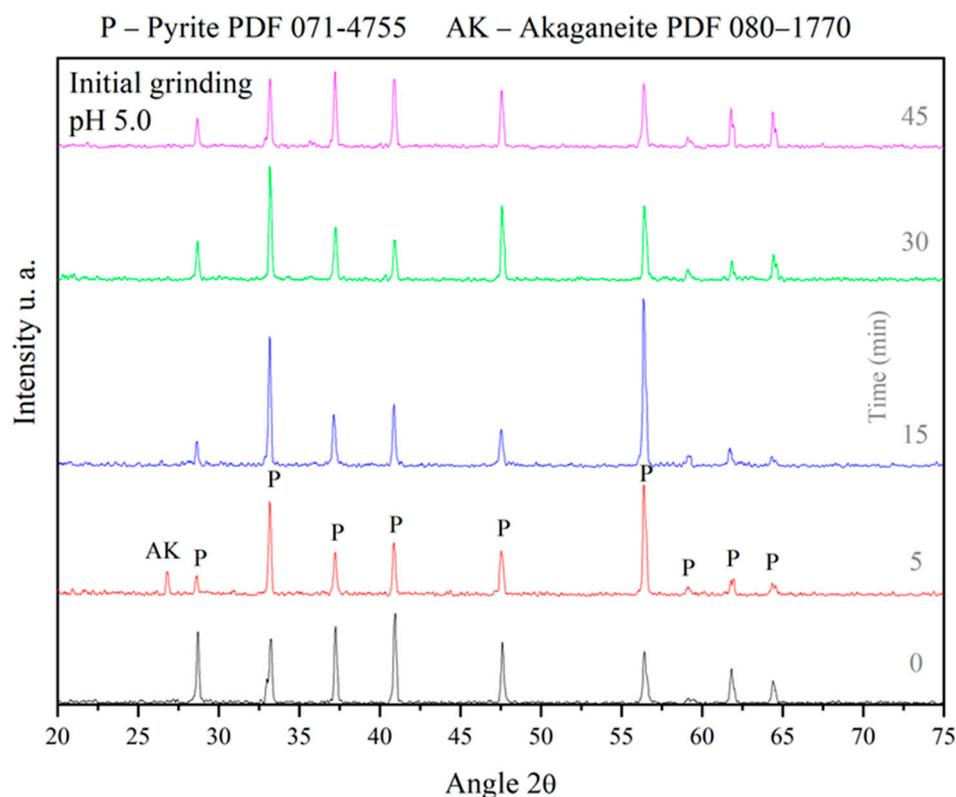
**Figure 4.** X-ray diffraction patterns of nonoxidised and oxidised pyrite obtained from grinding at an initial pH 5.0 and grinding times from 5 to 45 min.
