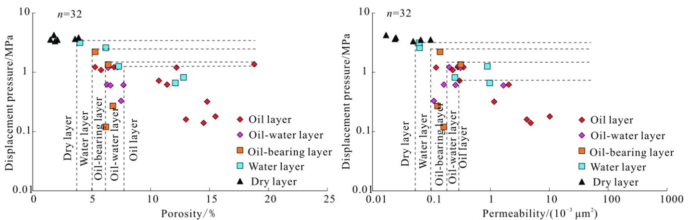
**Figure 8.** Displacement pressure vs. porosity and permeability for the volcanic reservoir in the Chepaizi Uplift.
