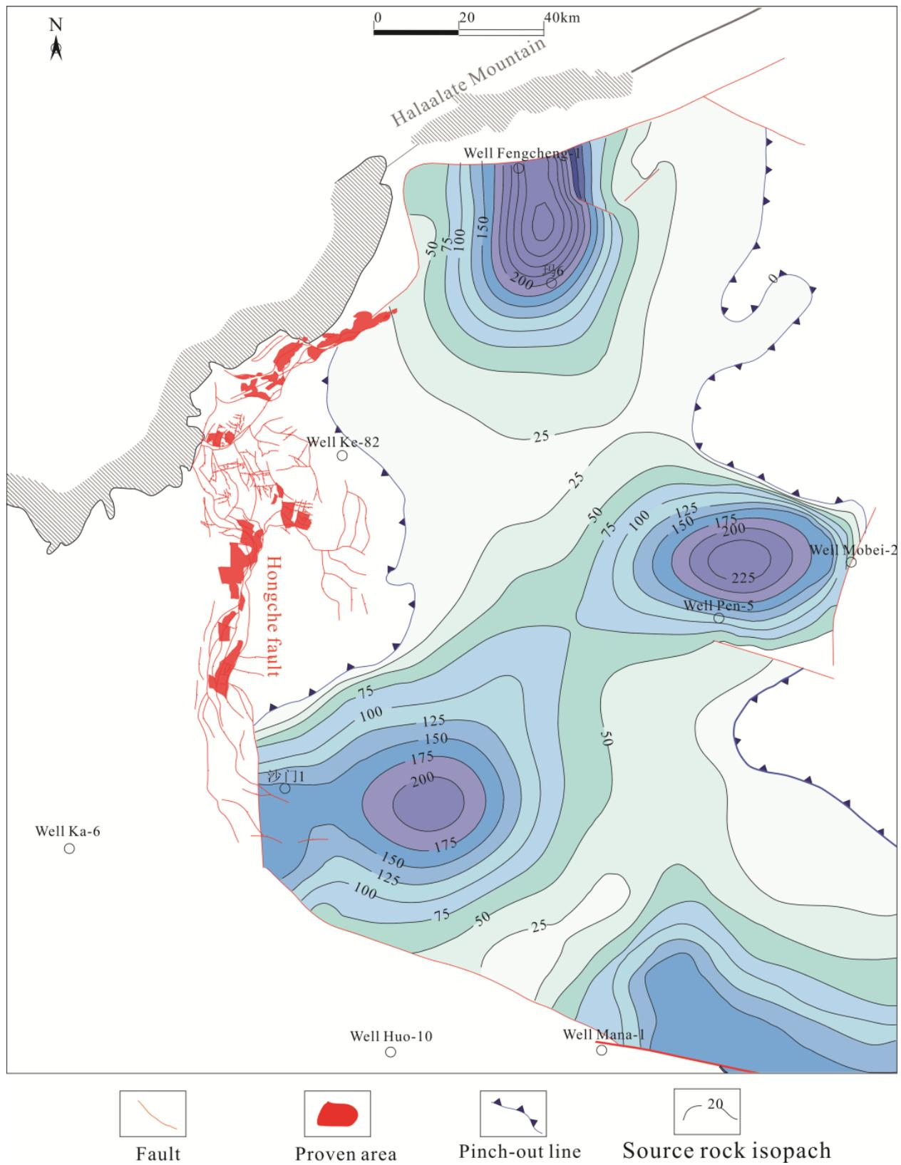
**Figure 5.** Distributions of the Permian Fengcheng Formation source rocks and faults in and around the Chepaizi Uplift.
