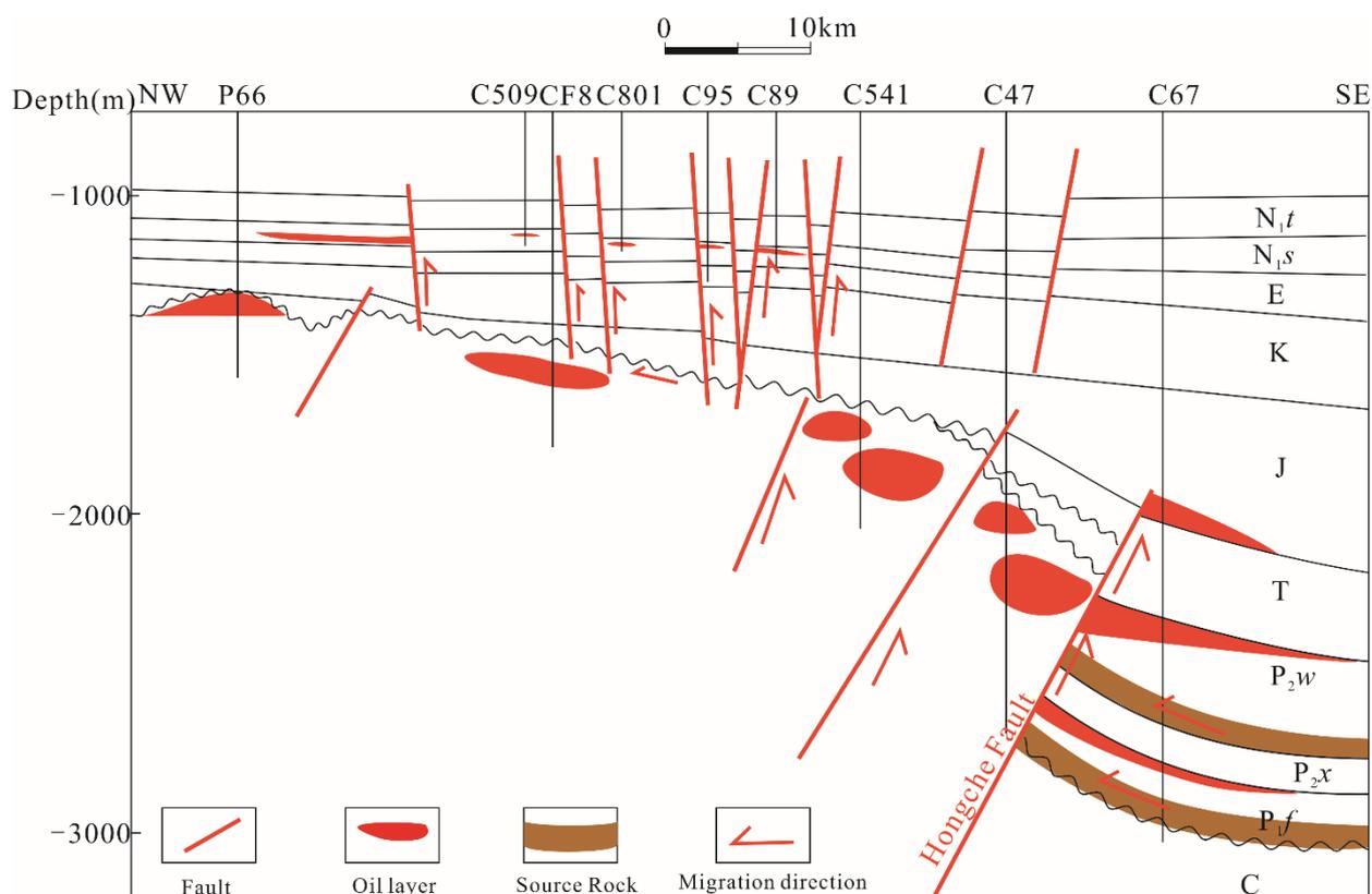
**Figure 11.** Hydrocarbon accumulation model of the Carboniferous volcanic rock reservoir in the Chepaizi Uplift.
