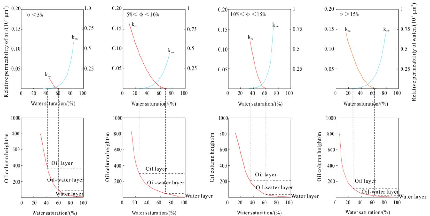
**Figure 9.** Correlation between reservoir physical properties and oil column heights of the Carboniferous reservoir in the Chepaizi Uplift.
