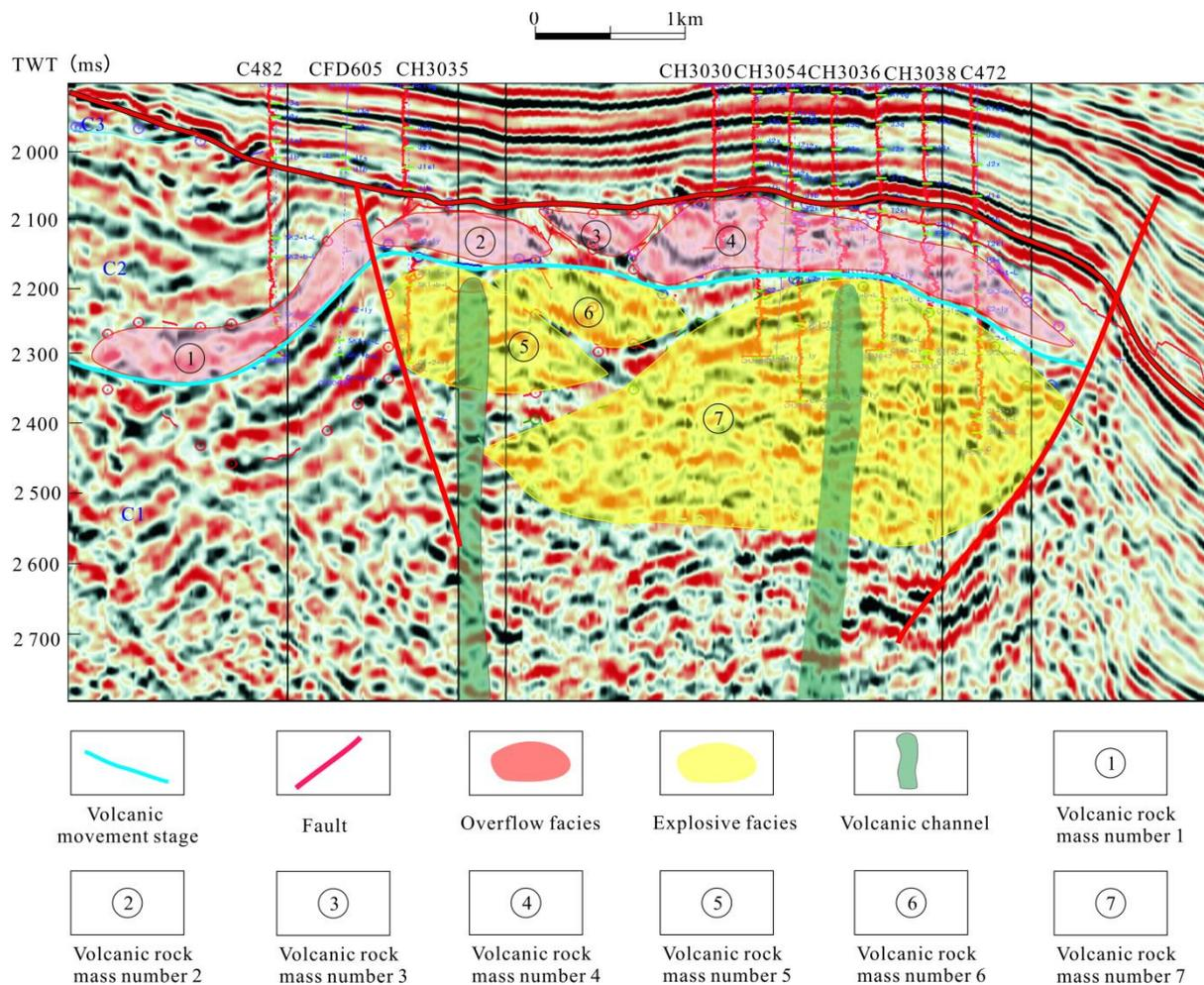
**Figure 3.** Distribution characteristics of volcanic rock bodies of the Carboniferous volcanic reservoirs in the Chepaizi Uplift.
