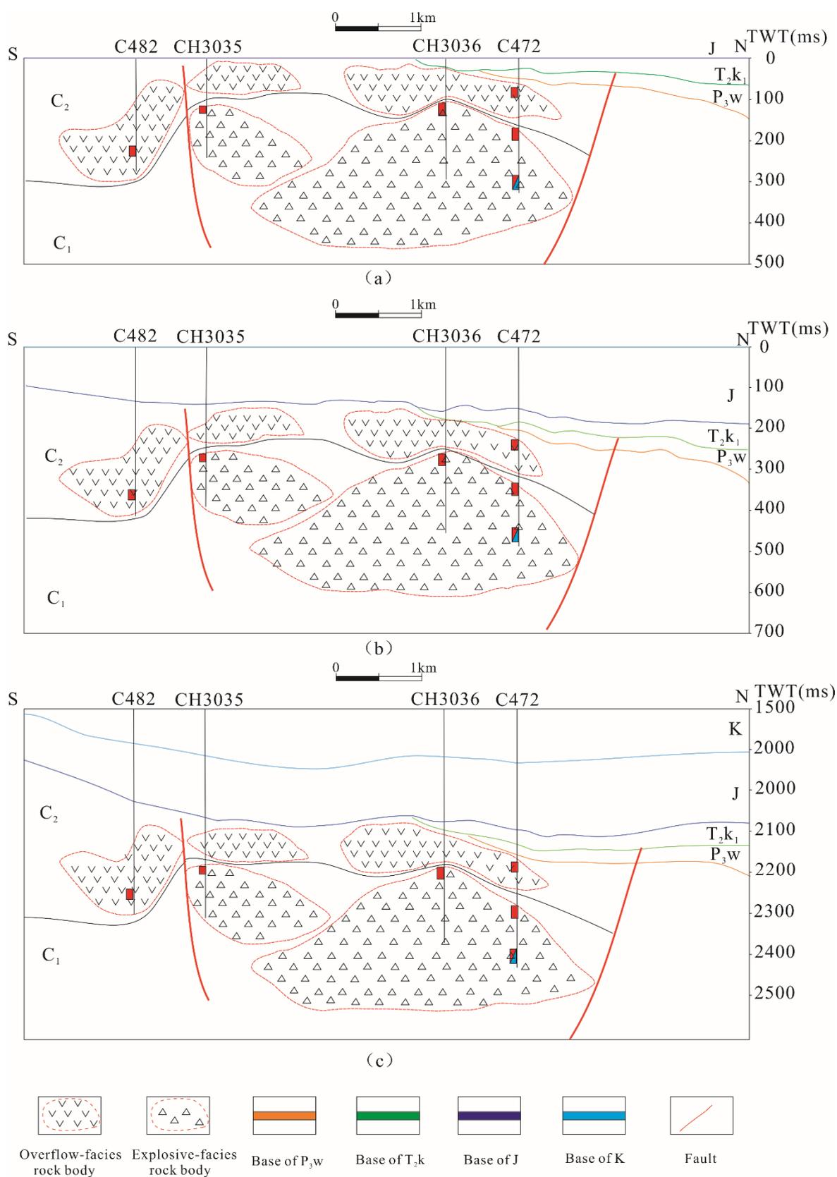
**Figure 7.** S-N profiles cross Wells C482-C472 in the Chepaizi Uplift, showing structural evolution. (a) The structural section of the flattening the Jurassic formation; (b) The structural section of the flattening the Cretaceous formation; (c) The present structural section.
