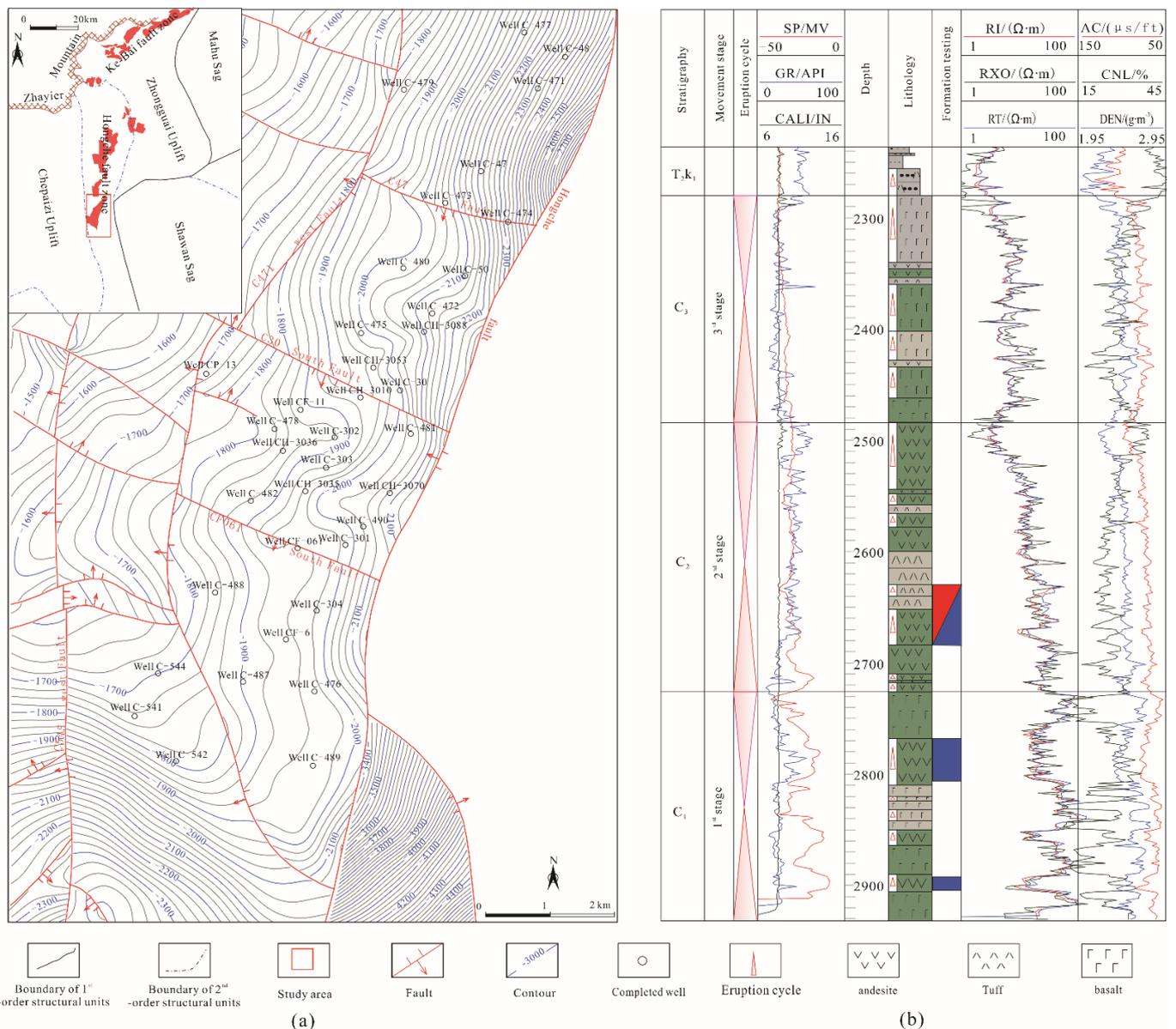
Figure 1. Structural position of the study area (a) and the stratigraphic column of the Carboniferous (b).
