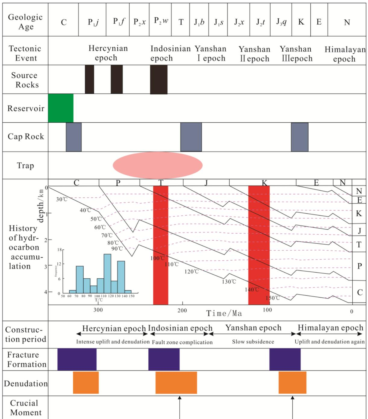
**Figure 10.** Hydrocarbon accumulation and evolution history of Carboniferous reservoirs in Chepaizi area.
