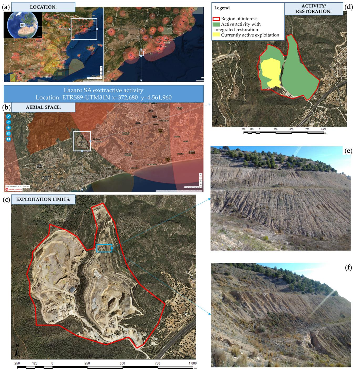
**Figure 1.** Location map of the limestone quarry studied. (a) General location of the study area in Catalonia, NE Iberian Peninsula. (b) Aerial space constrictions around the study area. (c) Exploitation limits and detail of the restored area. (d) Limits of the current extractive activity and limits of the restored areas. (e) Detail of the eroded slopes focused on the study. (f) Detail of the slope-berm restoration and erosion.
