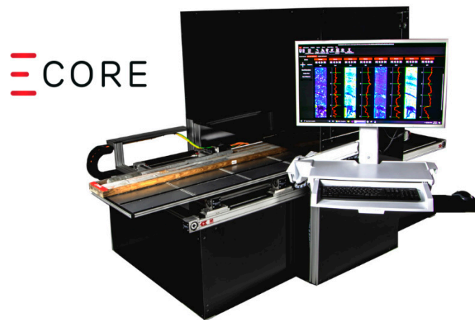
Figure 2. ECORE LIBS drill core scanner.
