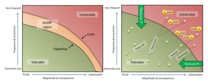
Figure 12. Schematic of ALARP principle applied in risk assessment [15].
