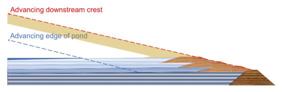
Figure 6. Schematic of the upstream raising of a tailings dam.
