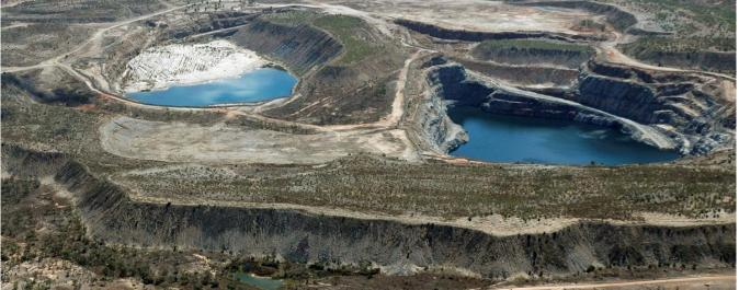
**Figure 23.** In-pit co-deposition of waste rock and thickened tailings (left-hand pit) at Kidston Gold Mines in north Queensland, Australia.
