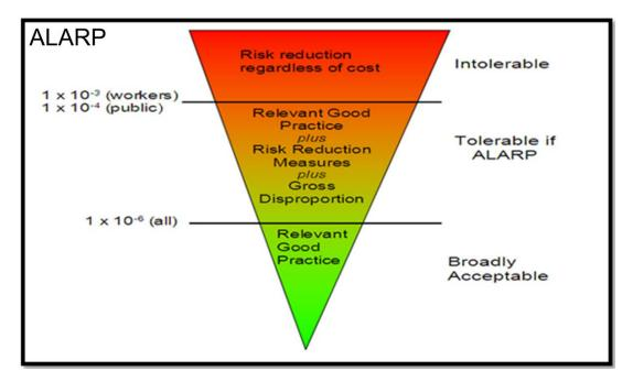
Figure 11. ALARP principle, including the probabilities of fatalities [14].
