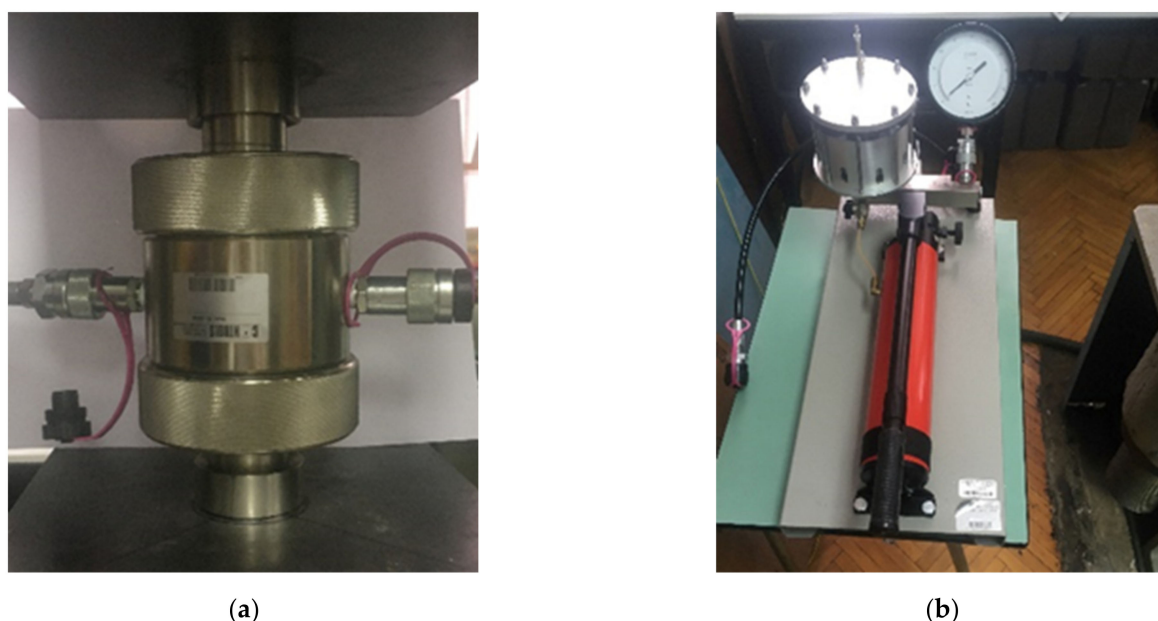
Figure 6. Triaxial test equipment: (a) Hoek cell and (b) manual confining pressure system for testing.
