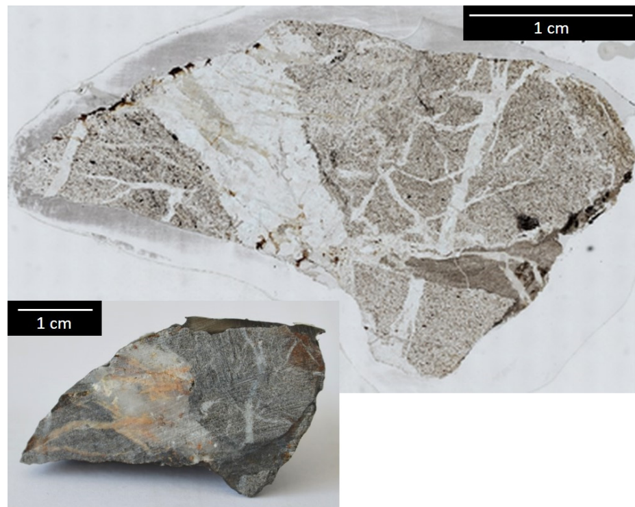
Figure 2. Main petrographic features of the studied sample. General view of the shale sample and of the thin section, on which the veins can be seen in white through the shale in grey (natural light).
