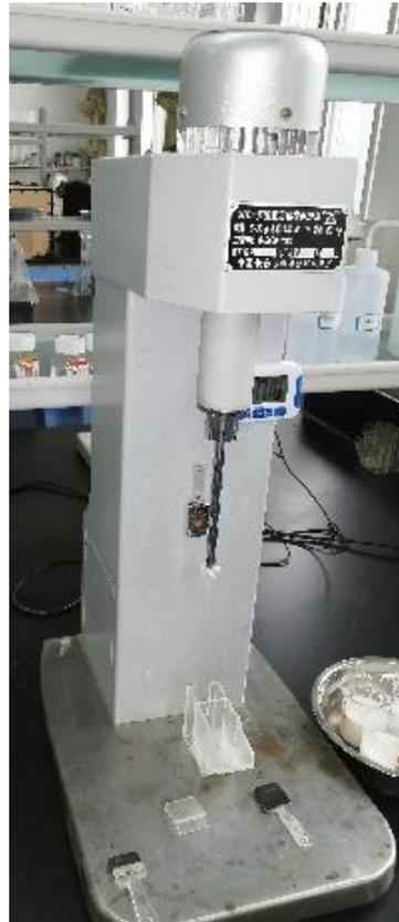
**Figure 2.** XFG–40 mL flotation machine with the flotation cell, dam board, and scraper.
