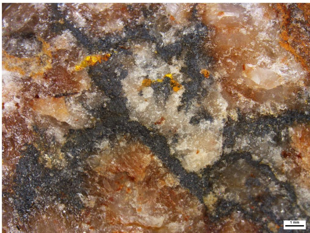
**Figure 2.** Irregular veinlets of U-Mo mineralization in limonitized quartz. The small cavities in the quartz are filled with a yellow uranyl molybdate—iriginite. Photo: Š. Ferenc.
