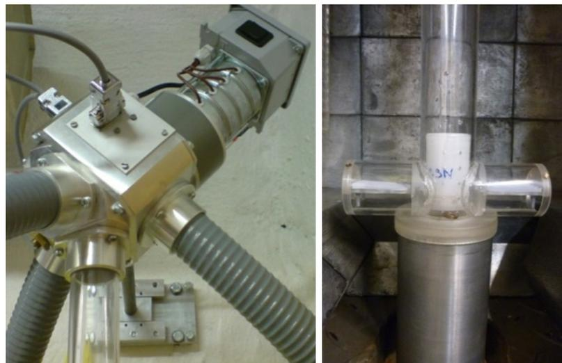
**Figure 2.** Components of the pneumatic tube delivery system installed at the MT-25 microtron. **Left:** 4-way routing head installed above the detector shielding with positions for sample insertion and delivery to the irradiation terminal (and back), counting position, and discarding position. **Right:** Sample in irradiation vial at the counting position on the detector inside the shielding.
