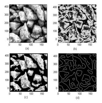
Figure 4. (a) Original image; (b) discretized image; (c) cropped image; (d) Canny application.
