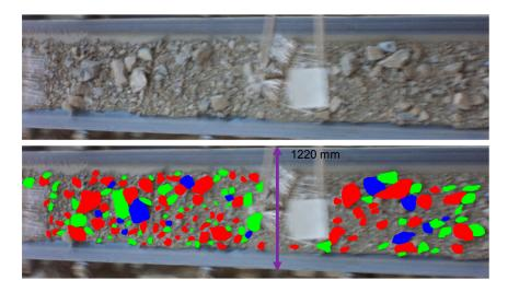
**Figure 13.** Manual marking on a conveyor belt (the width of the conveyor belt is represented in blue arrow).
