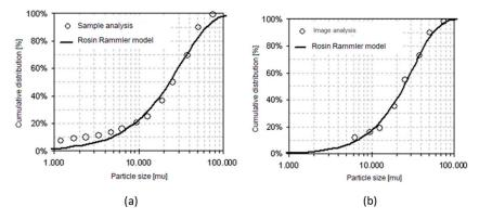
Figure 16. (a) Granulometric curves of samples. (b) Sensor curve. For images shown in Figure 15.
