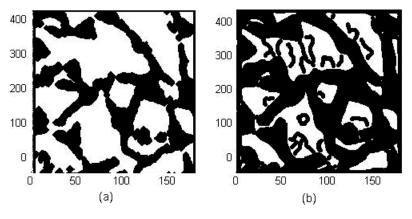
Figure 6. (a) Filled and eroded image; (b) binary image subtraction and Canny's dilated edge.
