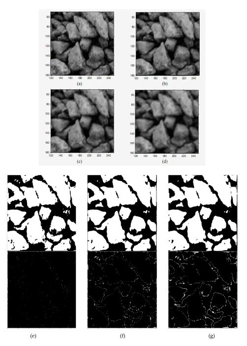
**Figure 2.** (a) Original image; (b) application of  $3 \times 3$  median filter; (c) application of  $9 \times 9$  Gaussian filter with  $\sigma = 1$ ; (d) application of  $9 \times 9$  average filter; (e–g) binarized images (using Otssu algorithm) and contour by subtraction of original image.
