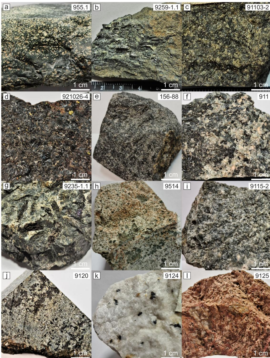
**Figure 2.** Photographs of the main rock varieties: (a) meimechite; (b) dunite with chromite schlier; (c) ore wehrlite; (d) ore pyroxenite; (e) kugdite; (f) ijolite-melteigite; (g) coarse-grained shonkinite; (h) alkaline microsyenite; (i) foyaite; (j) magnetite-apatite-diopside rock; (k) calcite carbonatite; (l) dolomite carbonatite.
