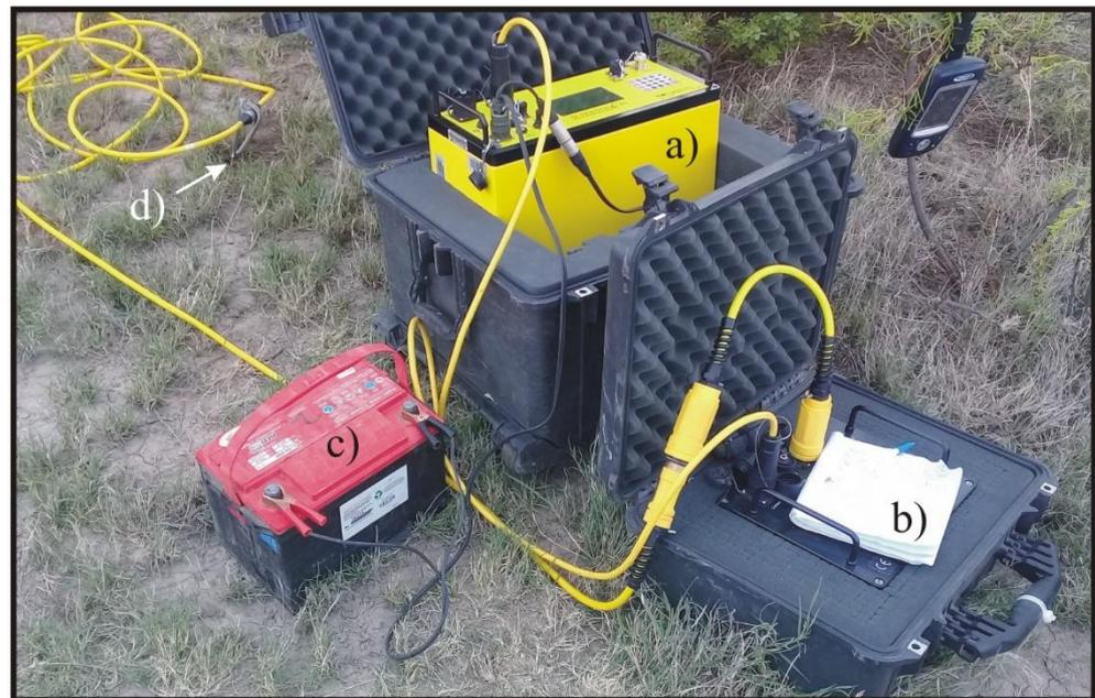
**Figure 2.** Data collection using the AGI SuperSting R1/IP/SP. (a) SuperSting™ console, (b) Switch box, (c) Battery, (d) Electrode.
