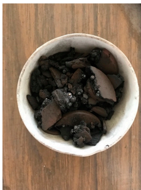
Figure 6. Cinder after 300 seconds, irradiation time at 0.6 kW, C/MBR 0.225 and 1 L/min nitrogen flow.
