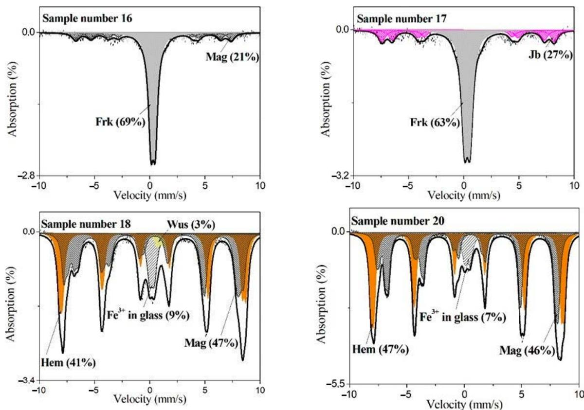
**Figure 14.** Mössbauer spectra obtained for steel dusts (No. 16, 17, and 18) and sinter dust (No. 20). Fitted subspectra, their assignments and contribution are visible on the spectra; Frk—franklinite, Hem—hematite, Mag—magnetite, Wus—wüstite, Jb—jacobsite. Absolute errors are estimated at  $\pm 1\%$  for components areas.
