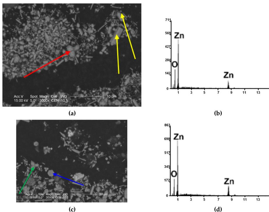
**Figure 8.** Dust from the Zn rectification process (sample No. 10): (a,c) SEM images: red arrow indicates zincite crystals forming twins; yellow arrows—single zincite crystals in the form of a column, sometimes with pyramidal ends; green arrow—twinning of columnar zincite crystals with pyramidal ends; blue arrow—hexagonal crystal of zincite; (b,d) the EDS spectrum.
