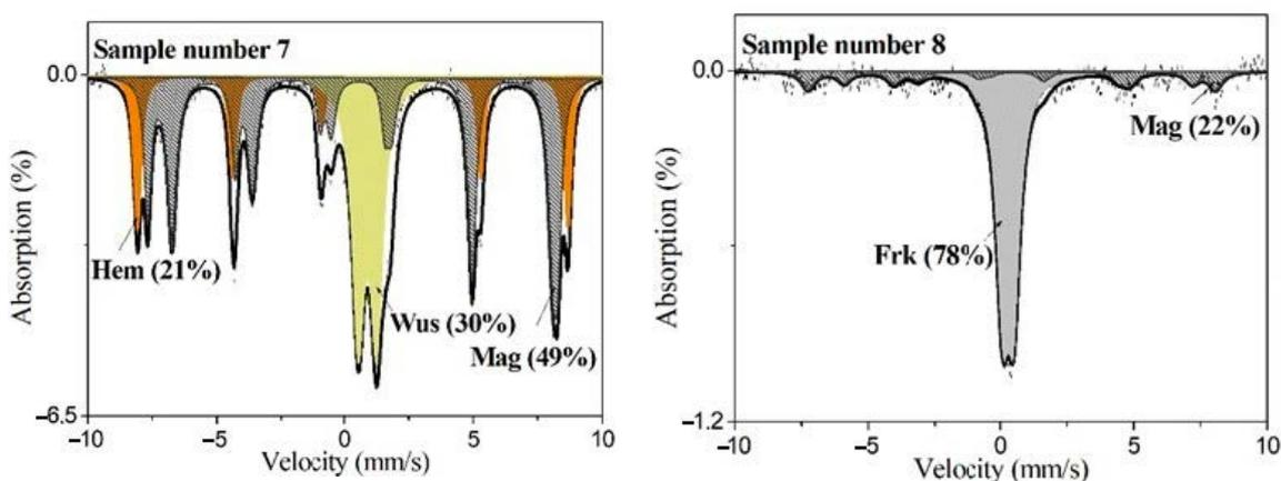
**Figure 13.** Mössbauer spectra obtained for scale (No. 7) and dedusting dust (No. 8). Fitted subspectra, their assignments and contribution are visible on the spectra; Hem—hematite, Mag—magnetite, Wus—wüstite, Frk—franklinite. Absolute errors are estimated at  $\pm 1\%$  for components areas.
