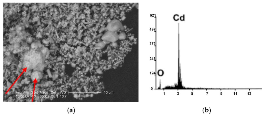
**Figure 10.** Particles from the zinc rectification process: (a) SEM image; the red arrows indicate components with the composition of cadmium oxides, probably monteponite CdO; (b) the XRD spectrum.
