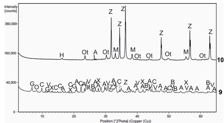
**Figure 9.** XRD pattern of sample No. 10 (Zn rectification) and No. 9 (sinter plant). Symbol explanation: A—anglesite, B—galena, C—challacolloite, G—gordaitite, M—monteponite, O—osakaite, Ot—otavite, V—matlockite, X—palmierite, Z—zincite.
