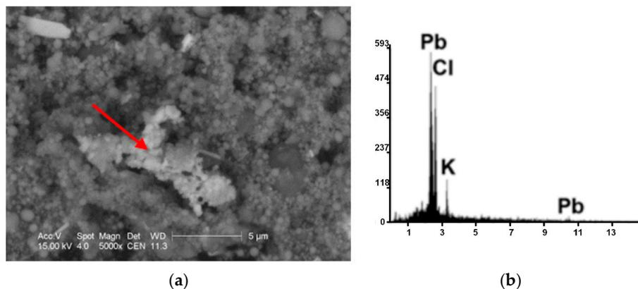
**Figure 12.** Dust particles from the sinter plant (sample No. 9): (a) SEM image; red arrow indicates a chalcocite  $\text{Cu}_2\text{S}$  aggregate; (b) the EDS spectrum.
