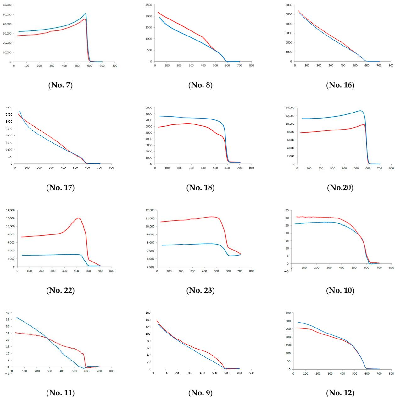
**Figure 16.** The  $k$ - $T$  curves ( $k$  ( $\times 10^{-5}$  SI units) is presented on the Y-axis and  $T$  (°C)—on the X-axis) of investigated dust samples. The heating lines are in red and cooling lines—in blue.
