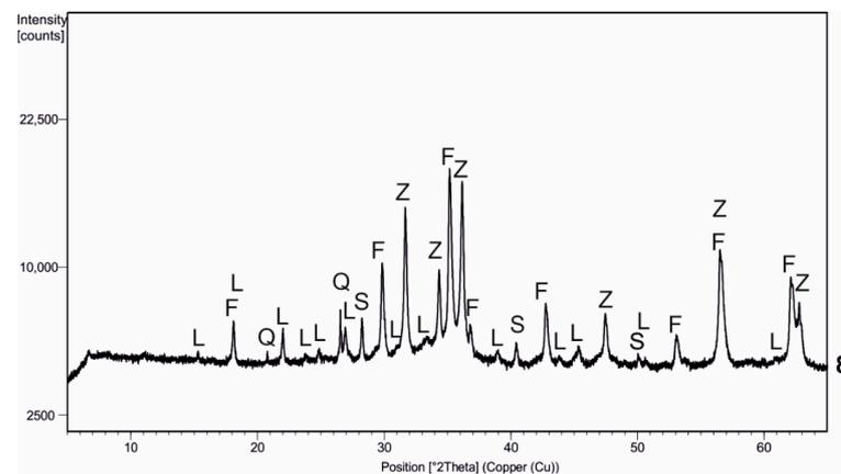
**Figure 4.** XRD pattern of de-dusting dust (sample No. 8). Symbol explanation: F—franklinite–jacobsite, L—laurionite, Q—quartz, S—sylvine, Z—zincite, M—magnetite.
