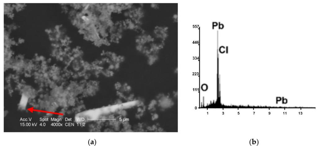
**Figure 3.** Laurionite particle in dust from de-dusting, sample No. 8: (a) SEM image (laurionite is indicated by a red arrow); (b) the EDS spectrum.
