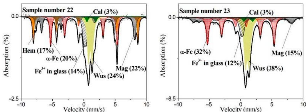
**Figure 15.** Mössbauer spectra obtained for iron-bearing sludges (No. 22, 23). Fitted subspectra, their assignments and contributions are visible on the spectra; Hem—hematite, Mag—magnetite, Wus—wüstite, Cal—calcite.
