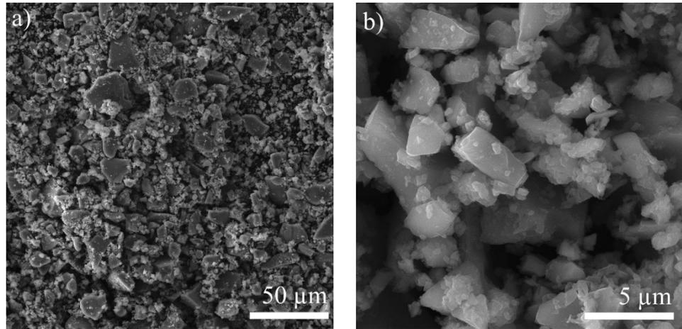
**Figure 4.** SEM images of milled Ecuadorian BMS in lower (a) and higher (b) magnifications.
