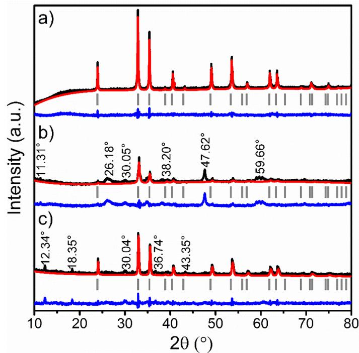
**Figure 3.** XRPD patterns of (a) milled BMS precursor, and (b) P-180 and (c) 180 powders, with the corresponding Le Bail refinements. Experimental pattern (black), calculated pattern (red) and difference plot (blue). Gray vertical bars correspond to IH-SS, PDF 01-070-8143.
