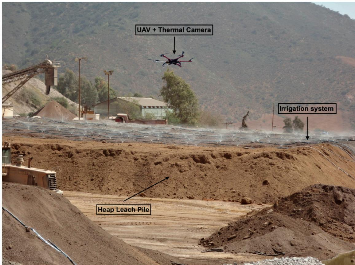
Figure 1. Setup implemented in the heap pile.
