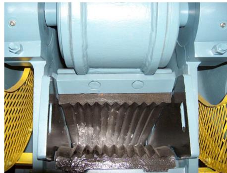
Figure 1. Jaw crusher to improve the grain shape.
