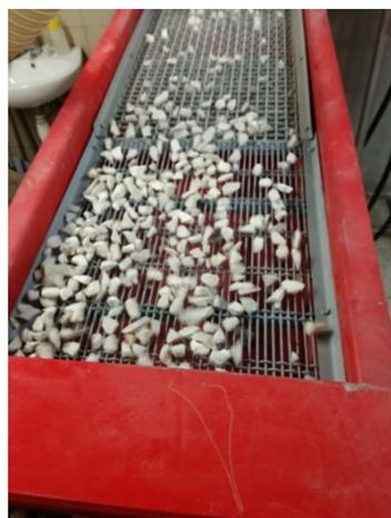
**Figure 18.** Screening process and production of regular particles on the three-deck vibrating screen.
