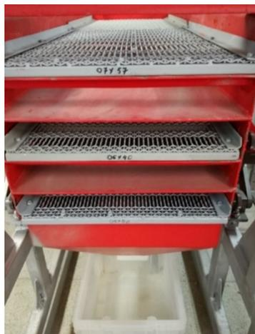
Figure 16. Screen decks and chutes after opening the screen head.
