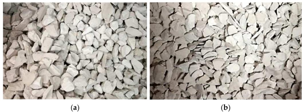
**Figure 20.** Limestone 12–14 mm, upper product, 99.3% regular particles, 10 mm × 60 mm screen (a), limestone 12–14 mm, lower product, 99.3% irregular particles, 7 mm × 60 mm screen (b).
