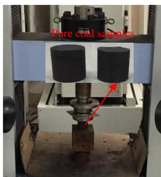
Figure 7. Short-term uniaxial creep tests on pure coal samples.
