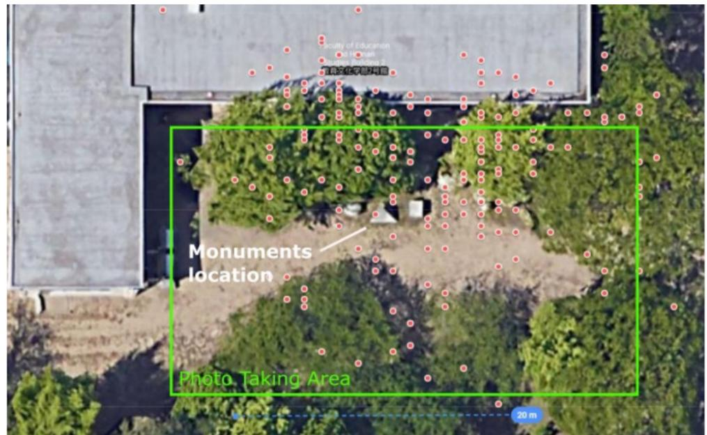
**Figure 13.** GNSS location of camera positions as logged by a smartphone (red dots) of the experiment on monuments of known dimensions.
