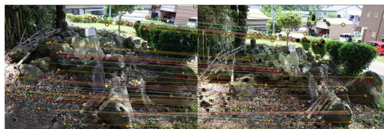
**Figure 7.** Keypoint matching tracks over two different views.
