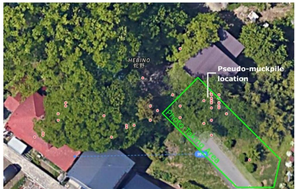
Figure 18. GNSS location of camera positions as logged by a smartphone (red dots) of the experiment on a pseudo-muckpile.
