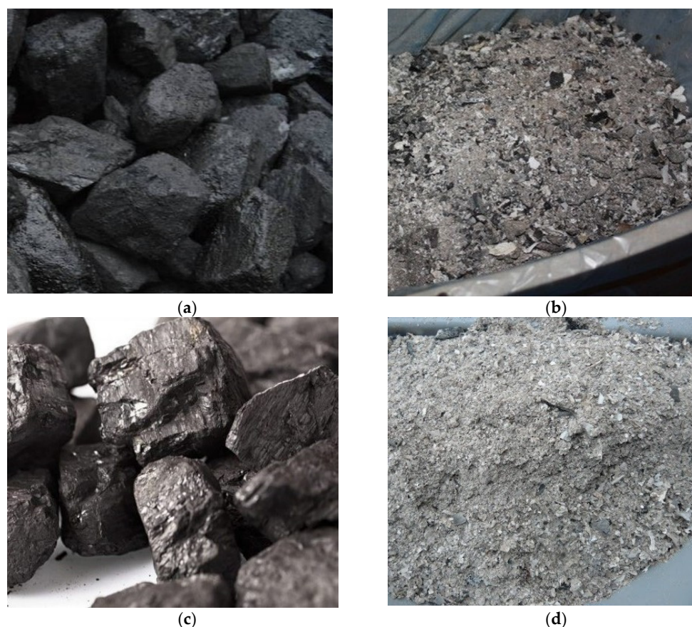
Figure 2. Research material: hard coal (a), ash from hard coal (b), eco-pea coal (c), and ash from eco-pea coal (d).
