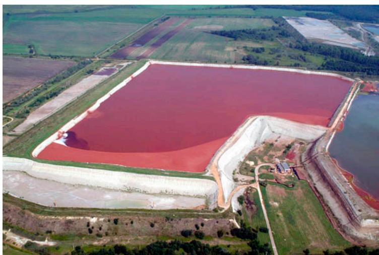
Figure 2. Planform of red mud (RM) yard disposed by damming stockpiling [2].
