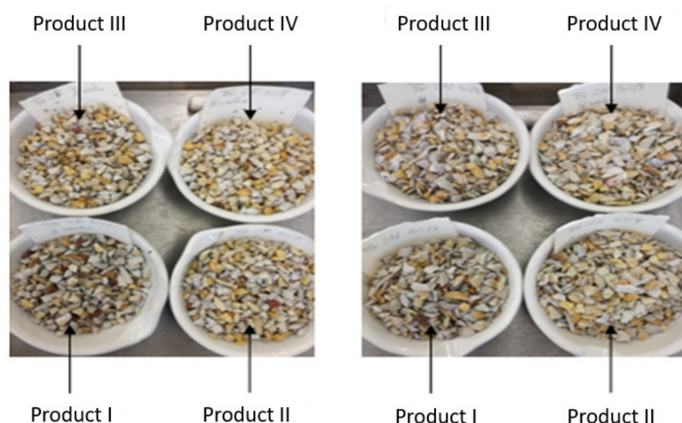
Figure 2. The exemplary chalcedonite product separated into four fractions for the regular particles (left) and irregular particles (right).
