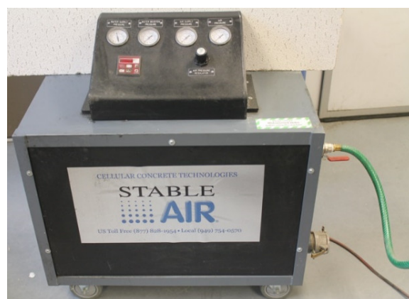
Figure 3. Stable Air ® model M100 foam generator.
