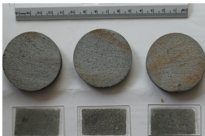
Figure 9. Thin sections of selected samples.
