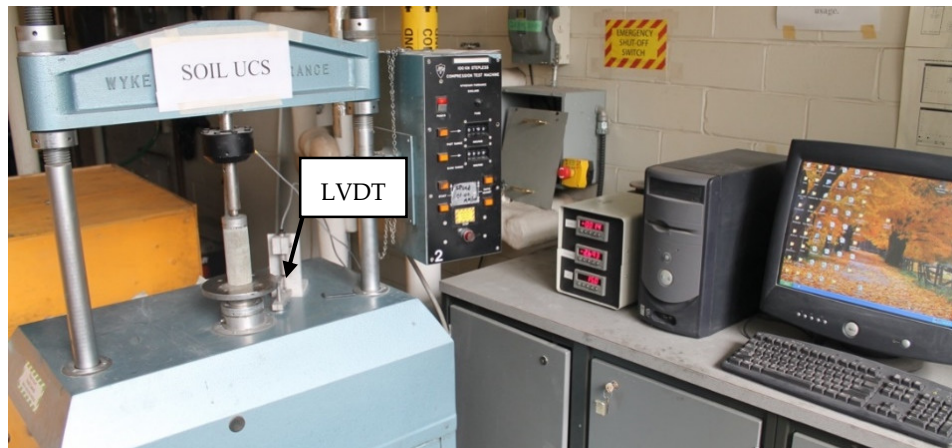
Figure 7. Experimental setup for unconfined compressive strength test showing linear variable displacement transducer (LVDT) for axial deformation measurement.
