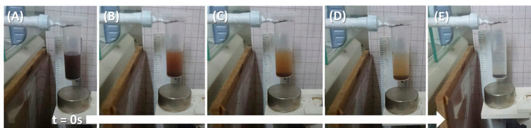
Figure 16. (A–E) Monitoring the magnetophoresis of NP@DTPA in the presence of a \text{Nd}_2\text{Fe}_{14}\text{B} magnet, as a function of time by means of an external weight device placed on the analytical balance pan (only the cantilever is shown) (adapted with permission from [43]).
