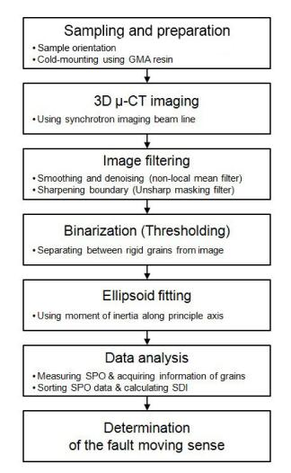
**Figure 2.** Flow chart showing the entire process of the newly developed 3D-shape preferred orientation (SPO) method to determine the fault motion sense. The method involves seven steps with from oriented sampling for SPO determination.
