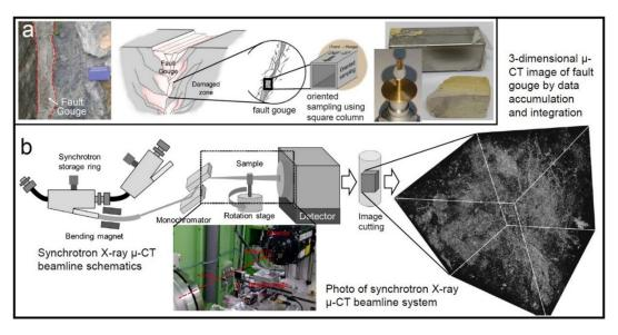
**Figure 3.** Schematic diagram of sampling and computational tomography (CT) imaging. (a) Photo of sampling site, oriented sampling process from the fault gouge in the fault zone, BK-1 sample, and sample cut to suitable size. (b) Schematic diagram showing the process of acquiring a 3D image of a sample from the 6C  $\mu$ -CT beamline at the Pohang Accelerator Laboratory.
