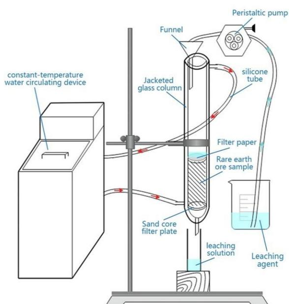
Figure 2. Column leaching apparatus.
