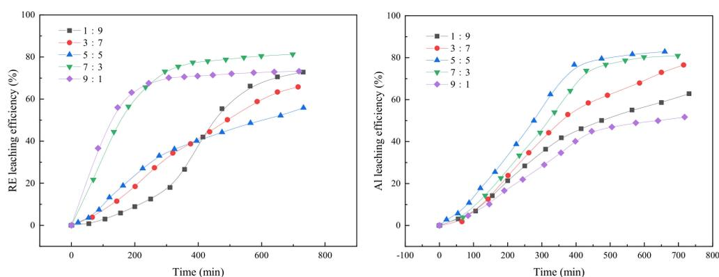
**Figure 4.** Effects of the molar ratio of leaching agent on the leaching processes of RE and Al.
