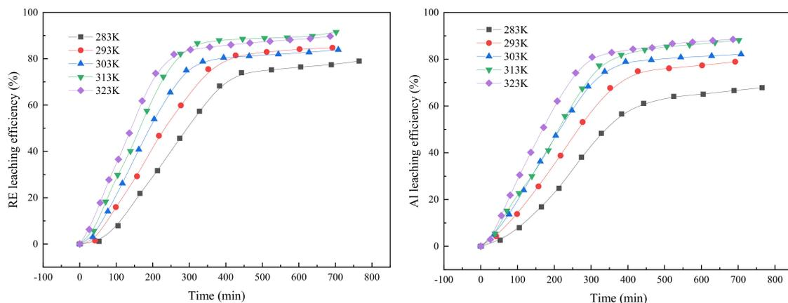
Figure 10. Effects of experimental temperatures on the leaching rate of RE and Al.
