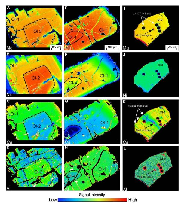
**Figure 6.** Representative electron microprobe (CPS) maps of the olivine grains. (**A–D**) olivine-1 grain with core of olivine-2 (see Figure 5B); (**E–H**)—olivine-1 with core of olivine-4 (see Figure 5D); (**I–L**)—olivine-3 grain. Elements, which distribution was mapped are specified on each inset.
