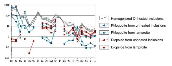
**Figure A1.** PM-normalized spider-diagram for compositions of clinopyroxene and phlogopite from olivine-hosted inclusions (SIMS data), the silicate rock matrix (LA-ICP-MS data) and the glasses of homogenized olivine-hosted inclusions (SIMS data).
