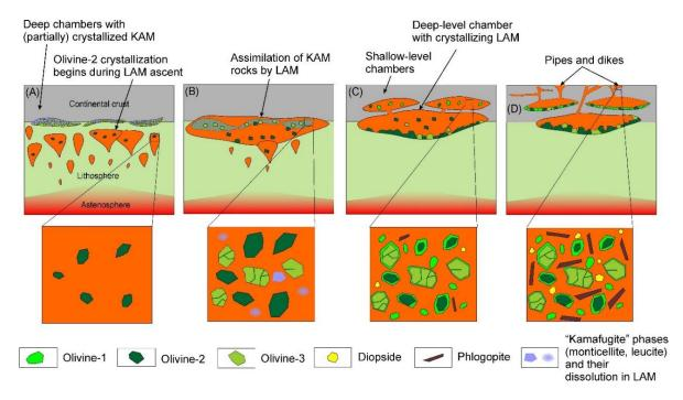
**Figure 14.** Schematic outlining processes of magma assimilation and the olivine crystallization sequence (types 1–3). (**A**) Uprise of a newly formed lamproite melt; (**B**) Accumulation of the lamproite melt in under-plated chambers and partial assimilation of cumulates, crystallized from a kamafugite-like melt; (**C**) crystallization of the resulting magma in deep- and shallow-level chambers; (**D**) emplacement of subvolcanic intrusions and ultimate solidification of the rocks.
