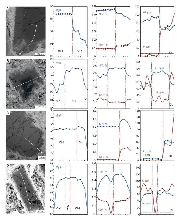
**Figure 5.** SEM BSE images and EPMA element profiles of olivine grains. (**A**) Olivine-2 with a rim of olivine-1. (**B**) Olivine-1 with an olivine-2 core. (**C**) Olivine-4 with a rim of olivine-1. (**D**) Olivine-1 with an olivine-4 core. White arrows on the SEM BSE images show compositional profile directions. Abbreviations: DL—detection limit, Ol—olivine.
