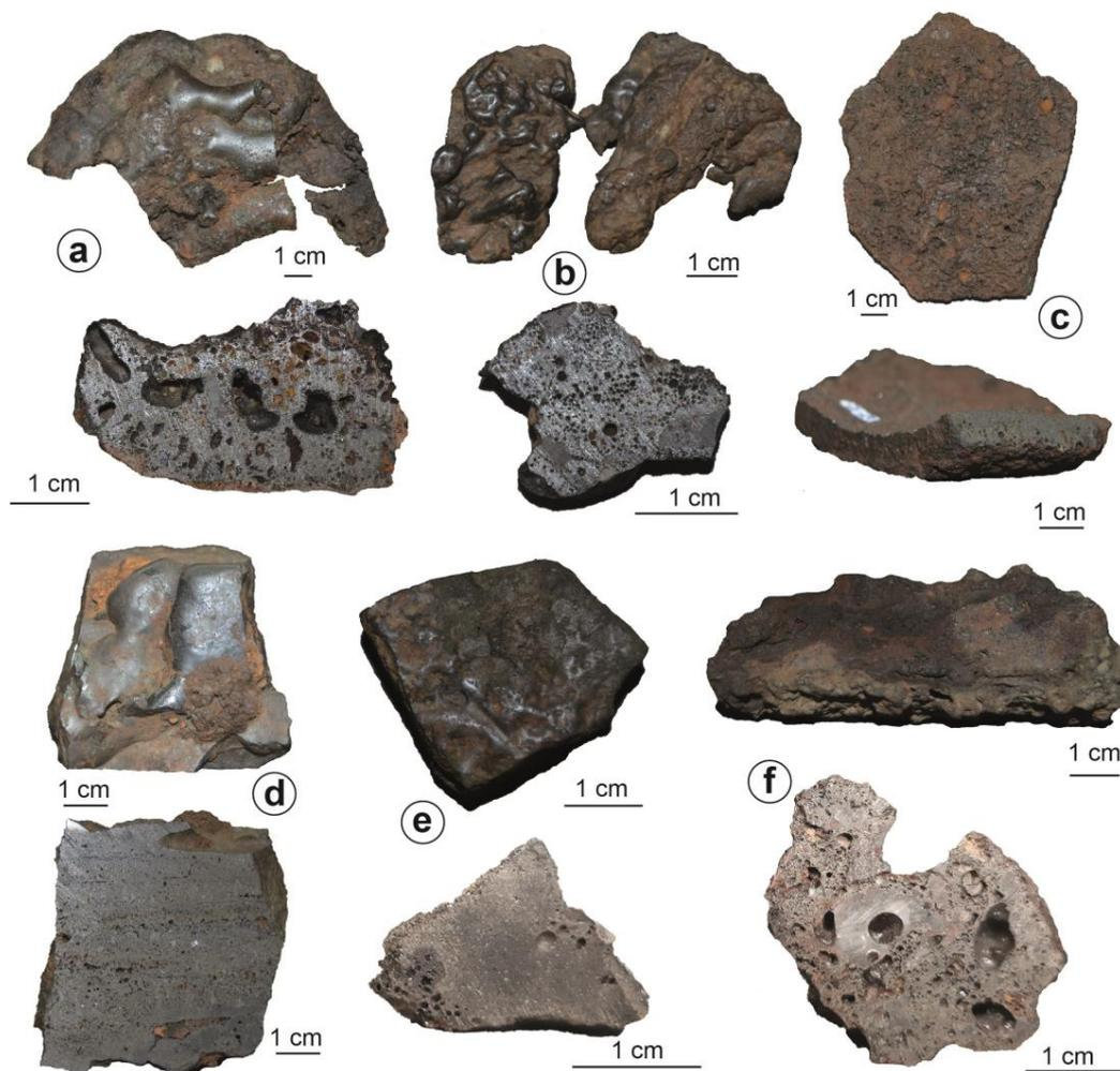
**Figure 2.** Photographs of representative samples of slags studied: (a) Group 1 very porous medieval slags, (b) Group 2 moderately porous medieval tap-slag, (c) Group 2 moderately porous medieval plano-convex slag. (d) Group 3 low porous medieval slag, (e) Group 4 low porous Roman slag. (f) Group 5 Roman cinder slag.
