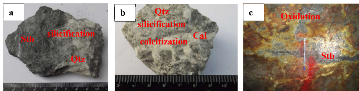
Figure 5. Typical alteration samples of the Lyhamyar antimony deposit. (a) Silicification with stibnite mineral; (b) silicification and calcitization with the limestone host rock; (c) oxidation on the stibnite ore. Abbreviations are as follows: Stb, stibnite; Qtz, quartz; Cal, calcite.
