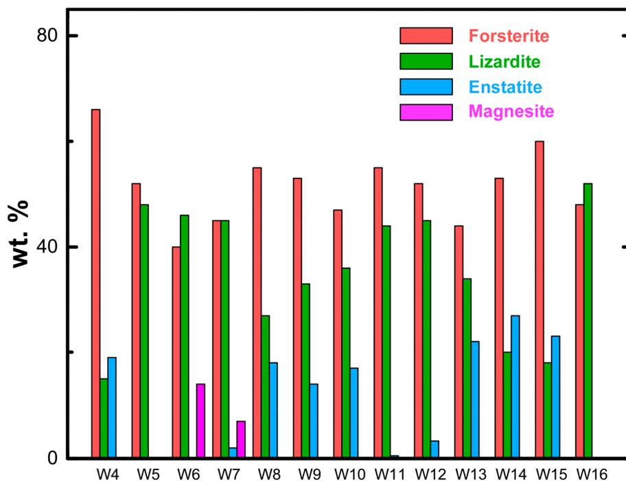
Figure 4. Mineralogical content (wt.%) of peridotite samples W4–W16.
