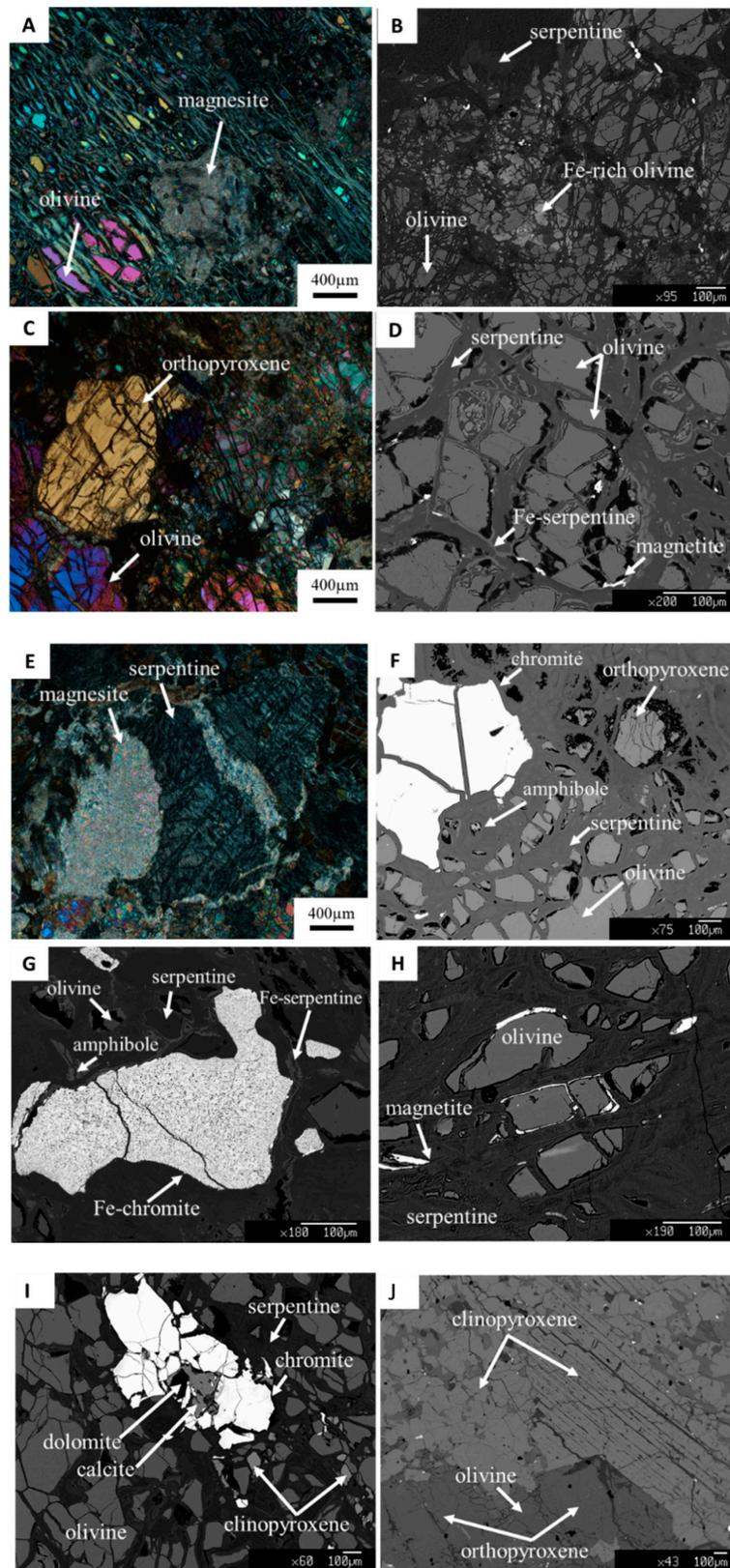
**Figure 5.** Optical microscopy (crossed polars; (A,C,E)) and back-scattered images (B,D,F–J) of serpentinized peridotites from the Rachoni mine (from samples W6, W13, W14, W15, W16).
