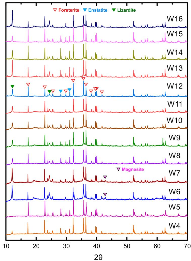
**Figure 3.** XRPD patterns of peridotite samples.
