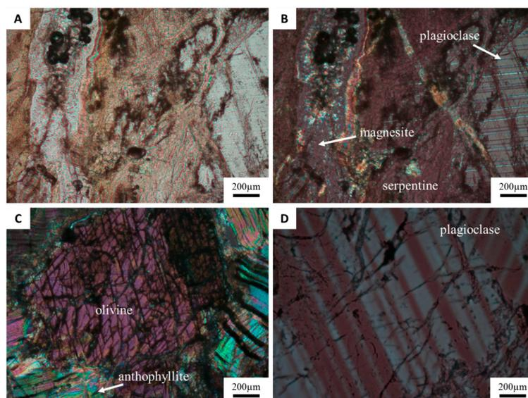
**Figure 7.** Optical microscopy (plane polarized light; (A); crossed polars; (B–D)) images of a clayey serpentinite with abundant plagioclase (sample W3); (A,B) magnesite vein cutting the serpentine matrix; (C) fractured olivine relic in contact with anthophyllite; and (D) plagioclase with twinning.
