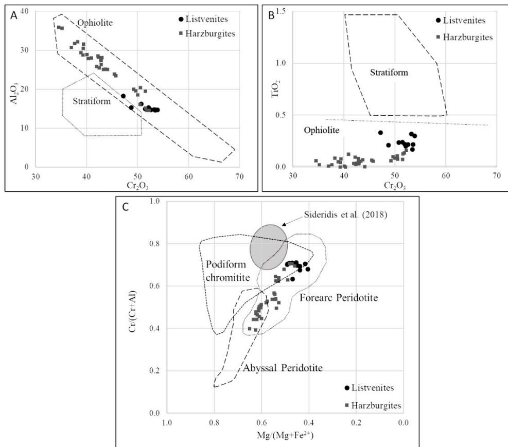
**Figure 9.**  $\text{Cr}_2\text{O}_3$  vs.  $\text{Al}_2\text{O}_3$  (A) and  $\text{TiO}_2$  (B) of the Rachoni peridotite chromites; (C)  $\text{Mg}/(\text{Mg}+\text{Fe}^{2+})$  vs.  $\text{Cr}/(\text{Cr}+\text{Al})$  of Rachoni peridotites chromite compared to chromitite chromites from the same area. Compositional fields for abyssal peridotites [25–27], forearc peridotites [26] and podiform chromitites [23,24,28] are shown for comparison.
