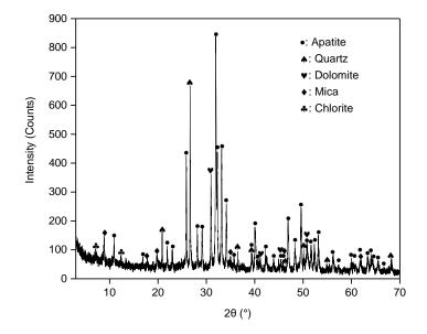
Figure 2. X-ray diffraction (XRD) phase analysis of Guizhou collophane ore.
