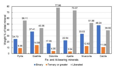
**Figure 11.** The total contents of each of the six minerals in the state of monomer liberation, intergrowth and inclusion.
