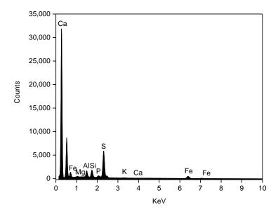
Figure 7. EDX spectra of pyrite.
