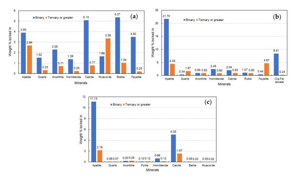
**Figure 9.** Intergrowth and inclusion contents between the Fe-bearing minerals and other minerals measured by MLA: (**a**) Pyrite; (**b**) Goethite; (**c**) Dolomite.
