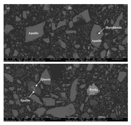
**Figure 3.** Dissemination characteristics of main mineral particles: (**a**) Apatite mineral; (**b**) Hornblende was included by apatite; (**c**) Apatite was included by quartz; (**d**) Pyrite mineral.
