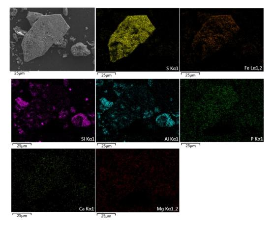
Figure 6. EDX elements mapping of pyrite.
