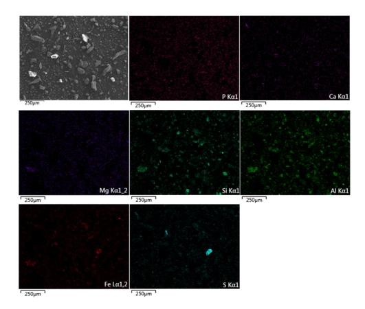
Figure 4. Energy dispersive X-ray spectrometry (EDX) elements mapping of collophane ore.
