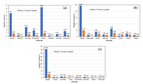
**Figure 10.** Intergrowth and inclusion contents between the Al-bearing minerals and other minerals measured by MLA: (a) Apatite; (b) Muscovite; (c) Calcite.
