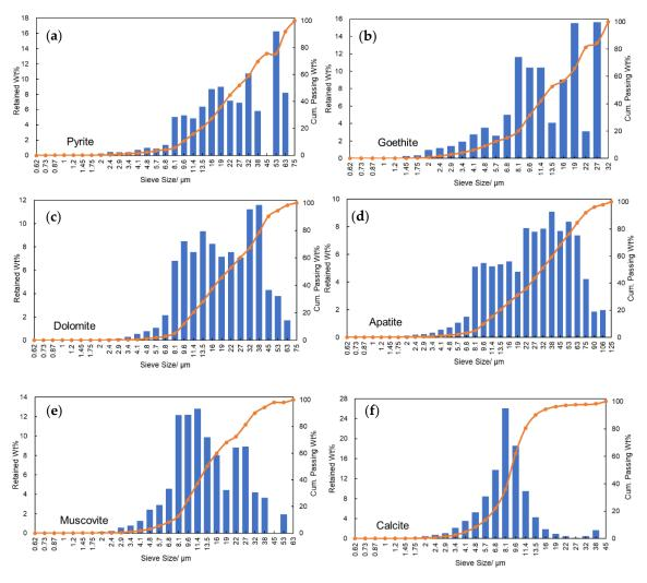
**Figure 8.** Grain size distribution of Fe, Al-bearing minerals: (**a**) pyrite; (**b**) goethite; (**c**) dolomite; (**d**) apatite; (**e**) muscovite; (**f**) calcite.
