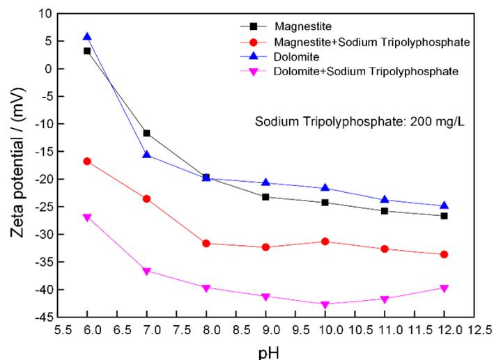
**Figure 9.** Zeta potential measurements for magnesite and dolomite with and without treatment of sodium tripolyphosphate.
