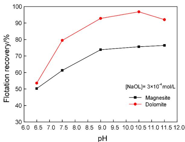
**Figure 4.** The influence of slurry pH on the flotation separation of magnesite and dolomite.
