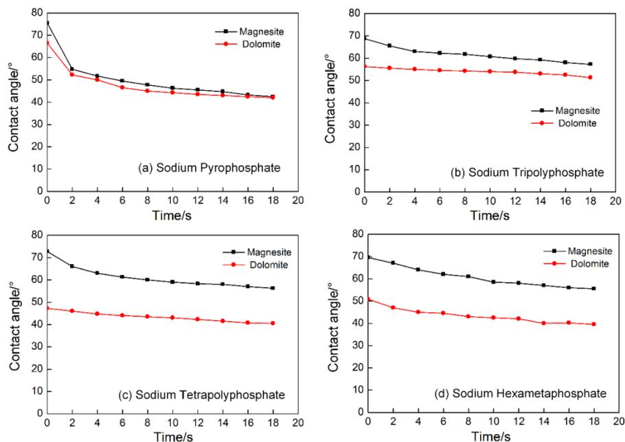
**Figure 7.** The relationship between contact angle and time under the effect of the sodium phosphate salts. Sodium Oleate  $3 \times 10^{-4}$  mol/L. (a) Sodium Pyrophosphate 300 mg/L, (b) Sodium Tripolyphosphate 200 mg/L, (c) Sodium Tetrapolyphosphate 100 mg/L, (d) Sodium Hexametaphosphate 4 mg/L.
