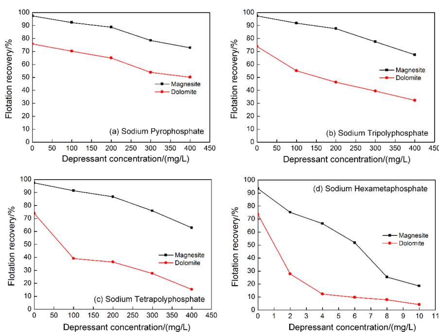
**Figure 5.** The influence of the concentration of phosphate with different chain lengths on the recovery of mineral flotation. Sodium Oleate  $3 \times 10^{-4}$  mol/L. (a) Sodium Pyrophosphate, (b) Sodium Tripolyphosphate, (c) Sodium Tetrapolyphosphate, (d) Sodium Hexametaphosphate.
