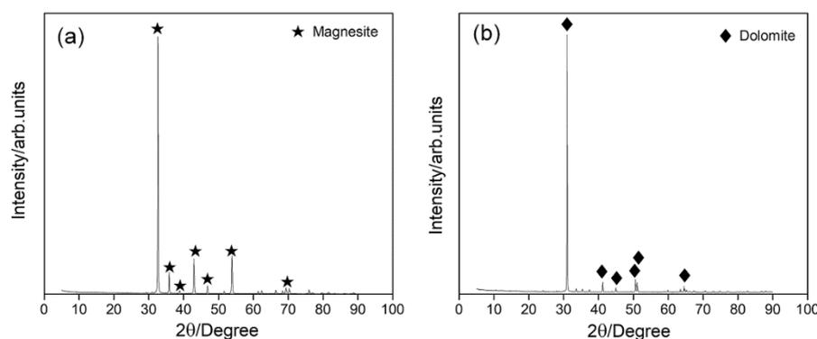
Figure 1. X-ray diffraction pattern of magnesite (a) and dolomite (b).
