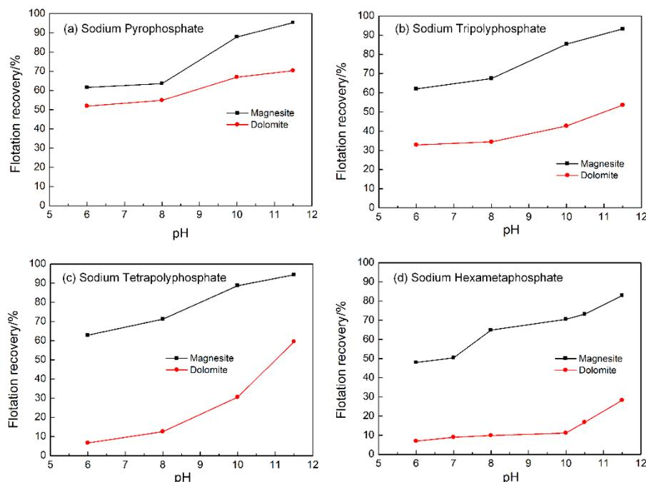
**Figure 6.** The effect of pH on mineral flotation recovery with different depressants. Sodium Oleate  $3 \times 10^{-4}$  mol/L. (a) Sodium Pyrophosphate 300 mg/L, (b) Sodium Tripolyphosphate 200 mg/L, (c) Sodium Tetrapolyphosphate 100 mg/L, (d) Sodium Hexametaphosphate 4 mg/L.
