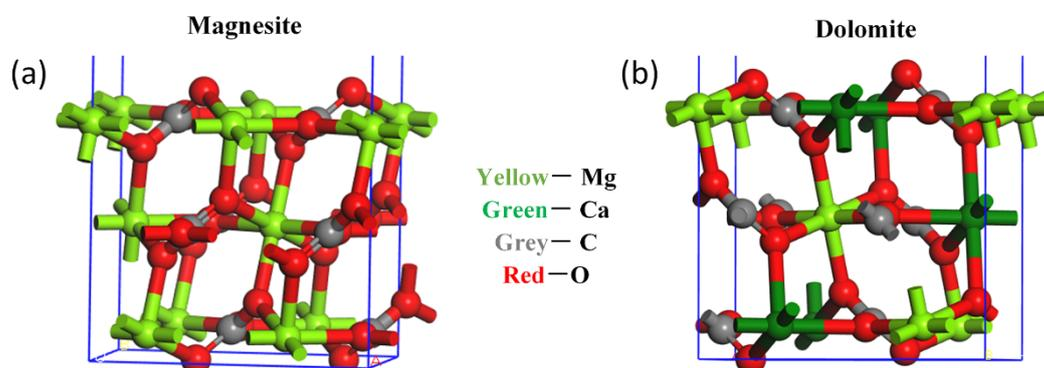
**Figure 10.** Structure diagram of common crystal cleavage planes of (a) magnesite and (b) dolomite.
