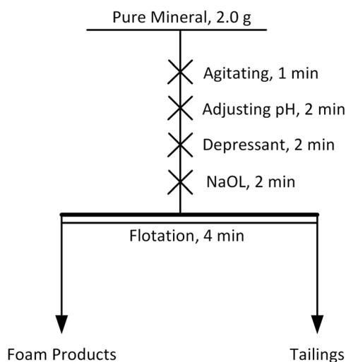
**Figure 2.** Flotation test flowsheet of pure minerals.
