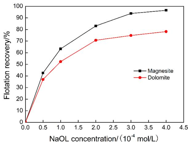
**Figure 3.** The effect of the concentration of collector on the flotation separation of magnesite and dolomite.
