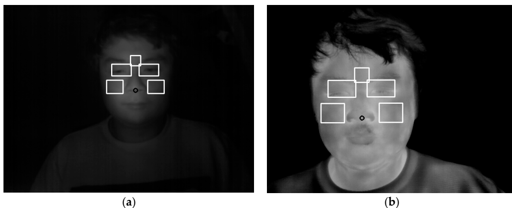
Figure 5. Symmetrical ROIs for FT measurement on thermal camera images determined by geometric transform matrix: (a) ROIs on NIR camera images; (b) ROIs on thermal camera images.
