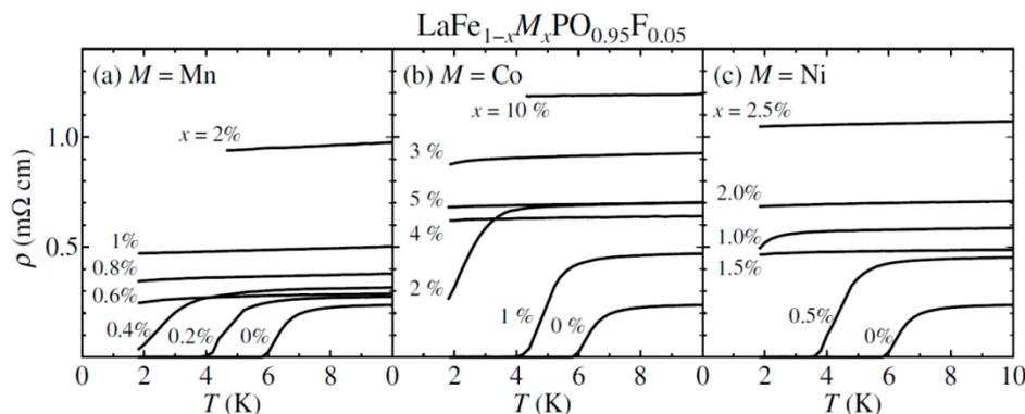
**Figure 2.** Temperature ( $T$ ) dependence of electrical resistivity ( $\rho$ ) for  $\text{LaFe}_{1-x}\text{M}_x\text{PO}_{0.95}\text{F}_{0.05}$  with various  $x$ s of (a)  $M = \text{Mn}$ ; (b)  $\text{Co}$  and (c)  $\text{Ni}$  below 10 K, respectively.
