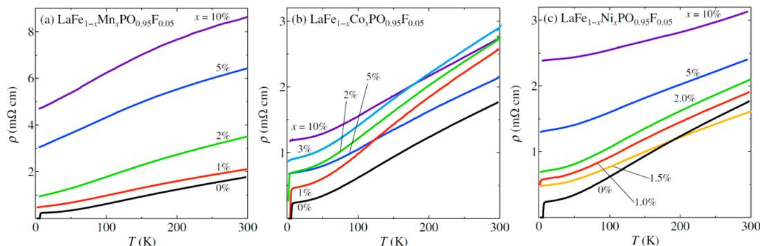
**Figure 1.** Temperature ( $T$ ) dependence of electrical resistivity ( $\rho$ ) for  $\text{LaFe}_{1-x}\text{M}_x\text{PO}_{0.95}\text{F}_{0.05}$  with various doping levels ( $x = 0\text{--}0.10$ ) of (a)  $M = \text{Mn}$ , (b)  $\text{Co}$  and (c)  $\text{Ni}$  in the wide  $T$ -region of  $T < 300$  K. The scale of the vertical axis of panel (a) is different from the others.
