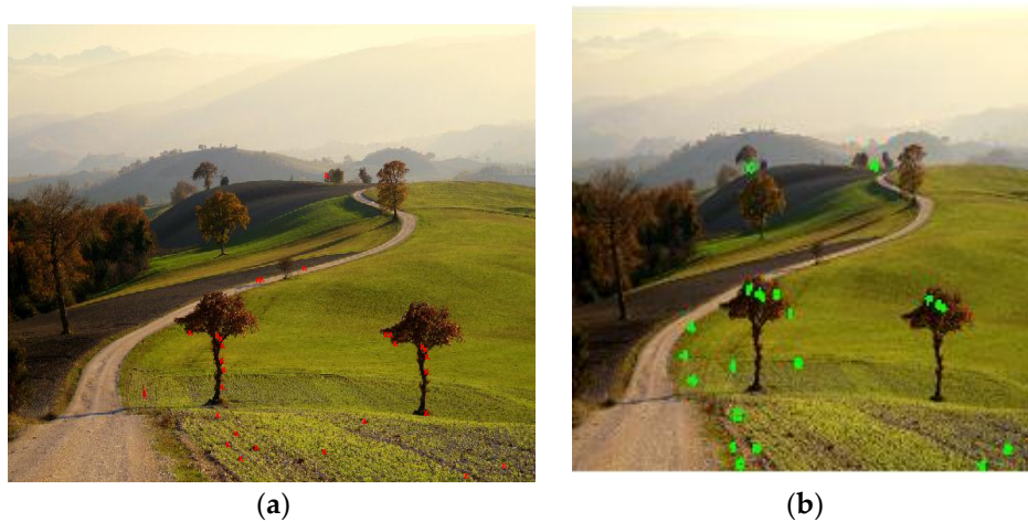
Figure 4. Centroids and Harris corners of image regions. (a) Centroids of image regions represented in red; (b) Harris corner points around centroids represented in green.
