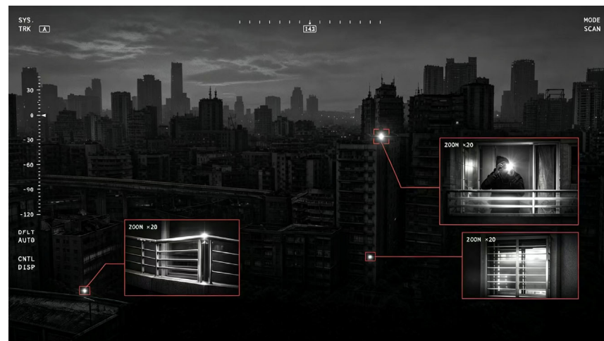
Figure 1. Illustrative urban laser active detection scenario based on the cat-eye effect. A hand-held optoelectronic device (e.g., a camera) in the sensor's field of view returns a strong, localized highlight echo along the incident laser path (upper-right callout). Other architectural glints, such as metal railings and window glazing (lower callouts), illustrate the general false-alarm problem that motivates this work. The red boxes highlight the bright echoes and their corresponding enlarged views.
