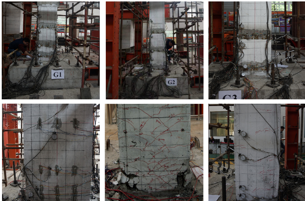
Figure 4. Representative damage evolution and terminal failure of the rectangular hollow-pier specimens.
