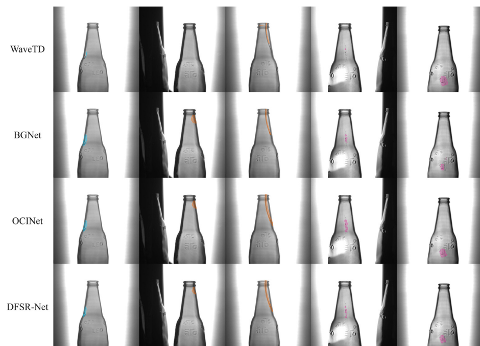
Figure 13. Qualitative comparison of segmentation results on the IGBD dataset. Each row shows the predictions of a different model, with cyan, orange, and purple masks representing bubble, crack, and stone defects, respectively.
