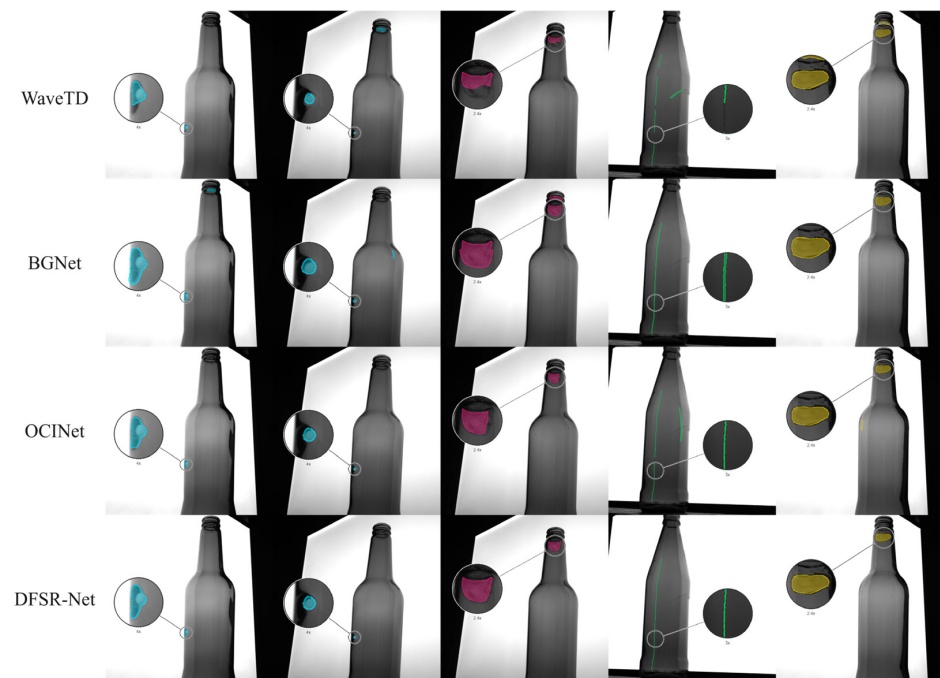
Figure 12. Qualitative comparison of glass bottle defect segmentation results on the public Bottle body dataset. Columns show two bubble examples, one inclusion, one stripe, and one deformation example, respectively. Rows show the predictions of WaveTD, BGNet, OCINet, and DFSR-Net. Cyan, magenta, green, and yellow represent bubble, inclusion, stripe, and deformation defects, respectively. Circular insets highlight local segmentation details and representative false-positive responses on normal bottle structures.
