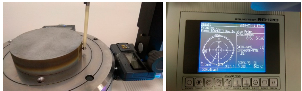
Figure 5. Measurement of macro-geometric deviations of circularity \Delta y_C of the eroded surface of symmetrically machined surfaces of experimental samples by the Roundtest RA-120 measuring device.
