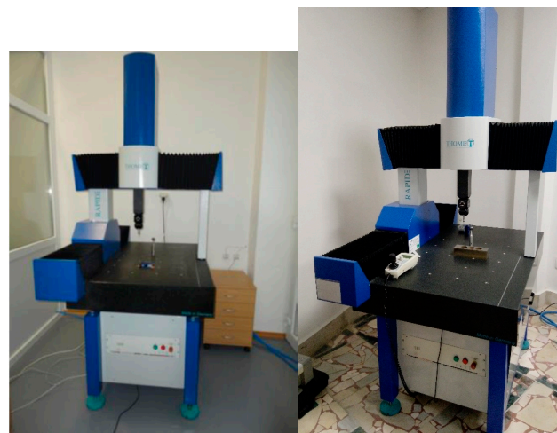
Figure 4. Measurement of macro-geometric deviations of the flatness of the eroded surface \Delta z_f of symmetrically machined surfaces of experimental samples by a 3D CNC coordinate machine Rapid-Plus.
