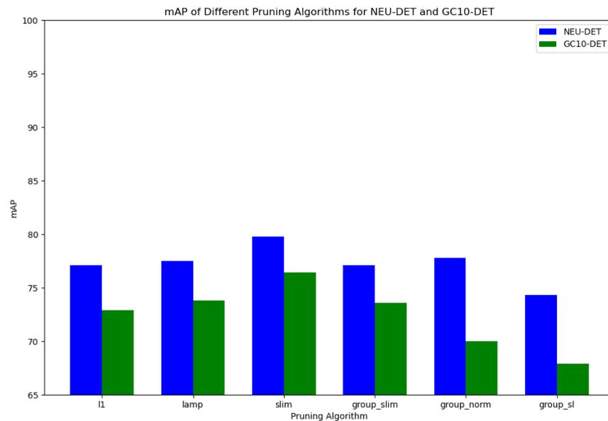
Figure 7. mAP of different pruning algorithms for NEU-DET and GC10-DET.
