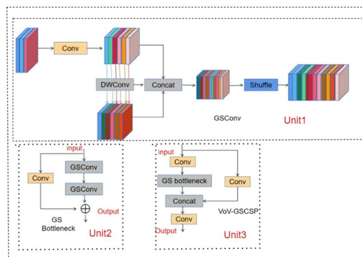
**Figure 3.** Structure diagram of GSConv and VOV-GSCSP lightweight modules.
