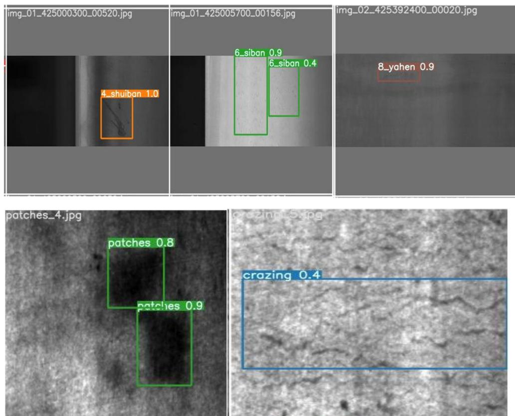
**Figure 10.** Part of steel strip defect detection results.
