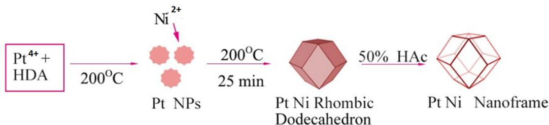
**Figure 10.** Schematic illustration of the synthesis of the Pt-Ni dodecahedral nanoframe. Reprinted with permission from Ref. [62]. Copyright 2020 American Chemical Society.
