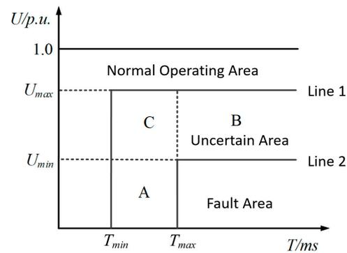
**Figure 1.** Uncertain region of sensitive load tolerance curve.
