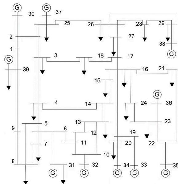
**Figure 3.** IEEE 39-node system architecture.
