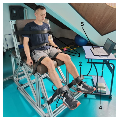
Figure 1. Testing setup. Participant in a custom-made chair (1: force transducer; 2: shanks; 3: rigid straps; 4: acquisition and analog-to-digital conversion unit; 5: monitor with visual feedback).
