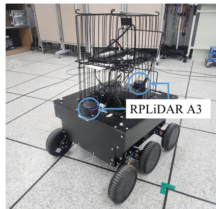
(a) Designed robot with two RPLiDAR A3 sensors
