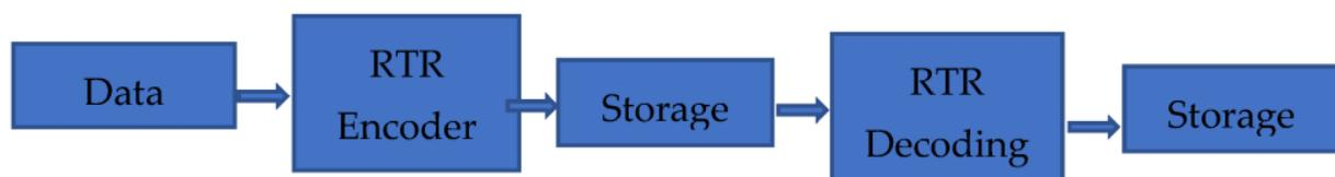
Figure 2. Block diagram of the removing temporal redundancy technique.
