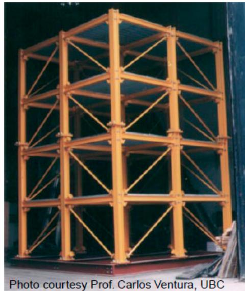
Figure 1. ASCE-SHM benchmark problem research structure prototype.
