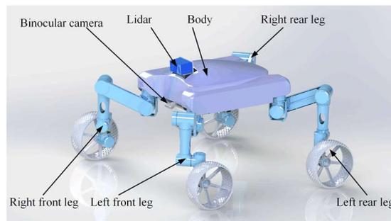
Figure 1. The whole structure of the wheel-legged robot.
